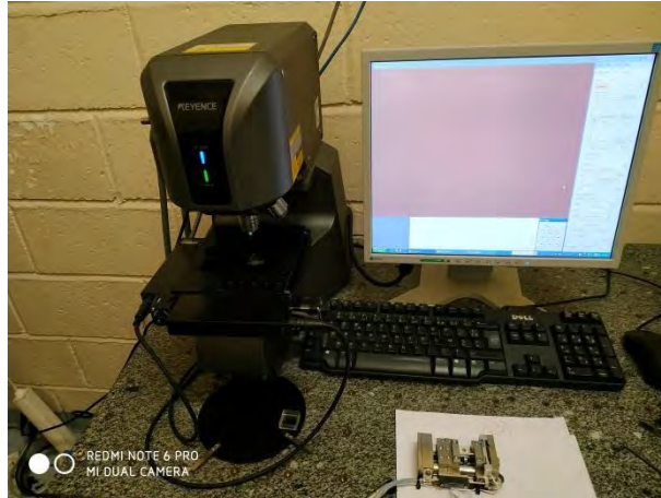
Figure 2.23 – KEYENCE confocal microscope coupled to the micro-tensile test DEBEN device.
