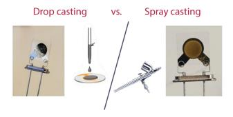
Figure III-2: Macroscopic results and visual inspection of the QCM resonators coated with the composite electrode – comparison between the drop casting and spray coating techniques.
