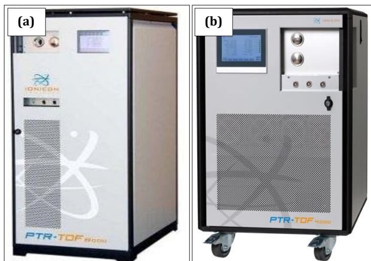
Figure II.19: Photo of PTR-ToF-MS (a) 8000 IONICON used at IMT Lille Douai and (b) 4000 IONICON used at UCLM.
