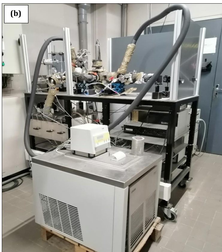
Figure II.10: (a) Schematic diagram and (b) photo of Cryocell and PLP-LIF system (El Dib et al., 2013).
