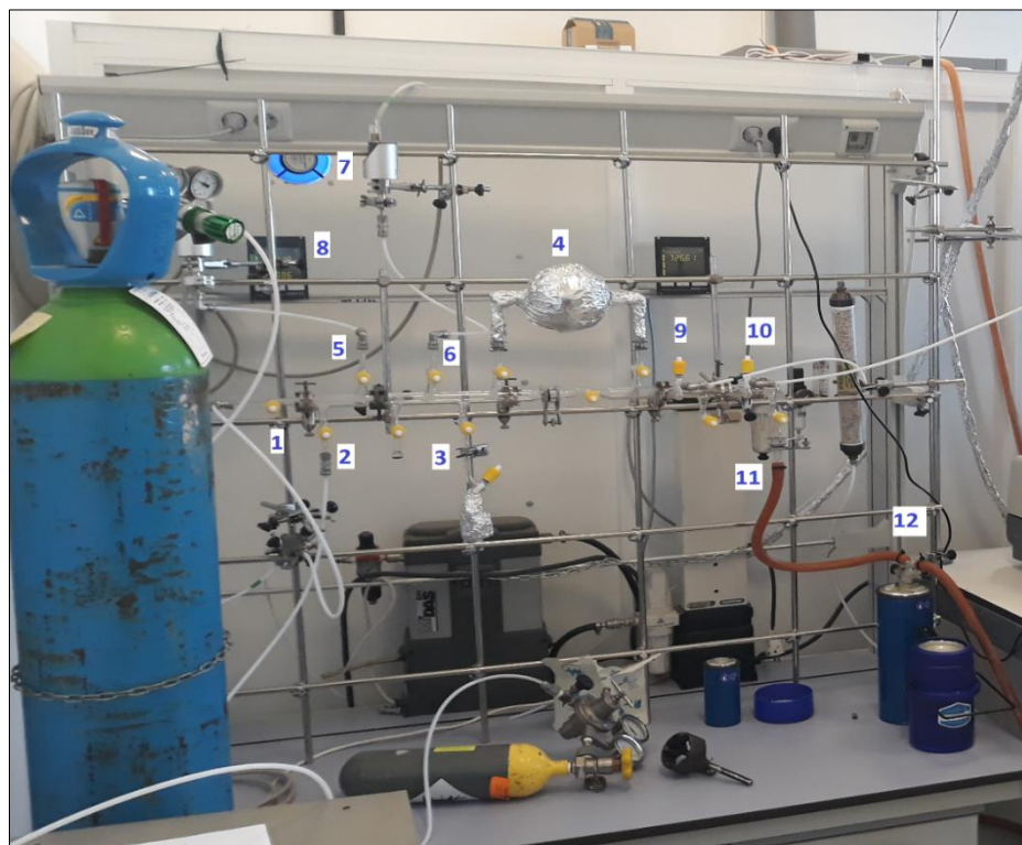
Figure II.6: Photo of the injection system of reactants used at UCLM.
