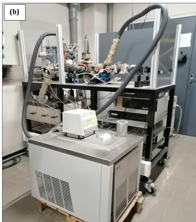
Figure II.10: (a) Schematic diagram and (b) photo of Cryocell and PLP-LIF system (El Dib et al., 2013).
