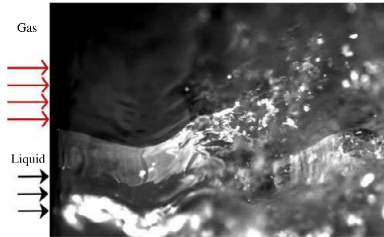
Fig. 1.7 – Primary wave of an air-water mixing layer. Extracted from Fuster et al. (2013).
