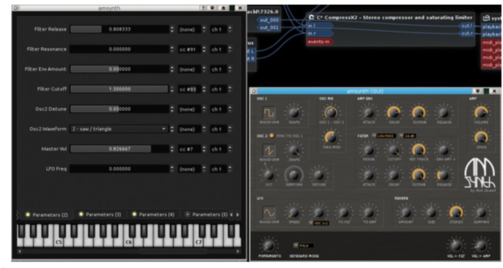
Figure 6.1.: Two possible graphical interfaces for the amSynth plugin 4 in the Carla host. On the left, the generic interface; on the right, the custom interface. Image from Linux Magazine Issue 175, June 2015.
