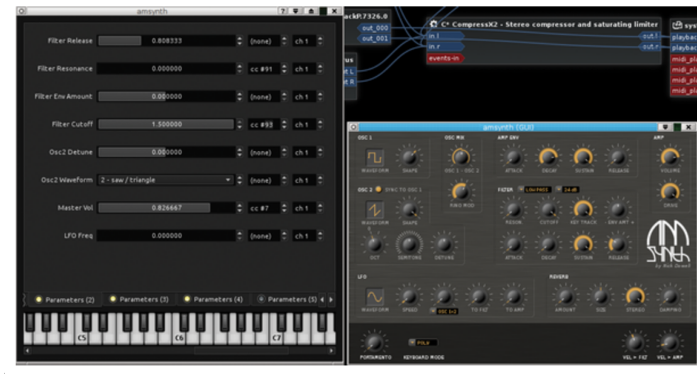
Figure 6.1.: Two possible graphical interfaces for the amSynth plugin 4 in the Carla host. On the left, the generic interface; on the right, the custom interface. Image from Linux Magazine Issue 175, June 2015.
