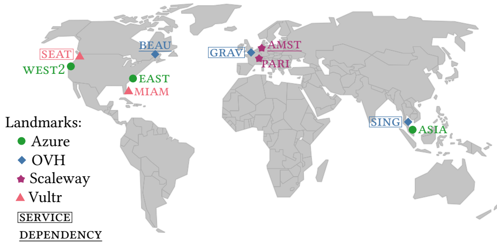
Figure 4.4 – Locations of landmarks and services in our multi-cloud experimental deployment. We deployed emulated clients in every location (region). The EAST, GRAV and SEAT landmarks were hidden during training.
