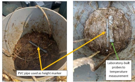
Fig S1. Interior part of the reactor showing the PVC pipes used as height indicator and the temperature probes to follow temperature
