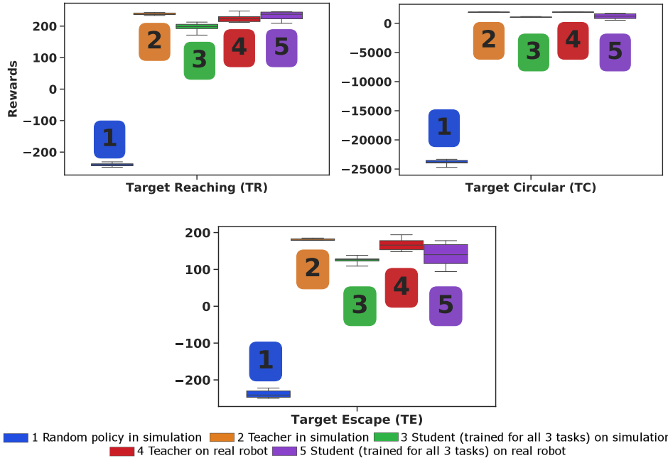
Figure 3.14: Main result: distillation in a continual learning setting of three teacher policies into a single student policy. The resulting policy is able to perform all three tasks both in simulation and in the real world, while minimizing forgetting.
