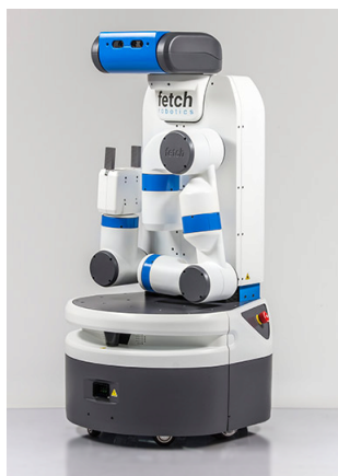
Figure 7.1: The Fetch robot, which allows navigation with a mobile base, and manipulation with its 10-DOF articulated arm. The robot has first-person embedded sensors (camera).
