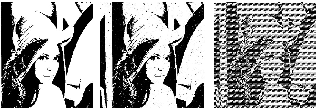
Figure 4.18: Transmitted Lenna, an SDF perspective when L_c = 128 chips, N = 4 , SNR = 11\text{dB}
