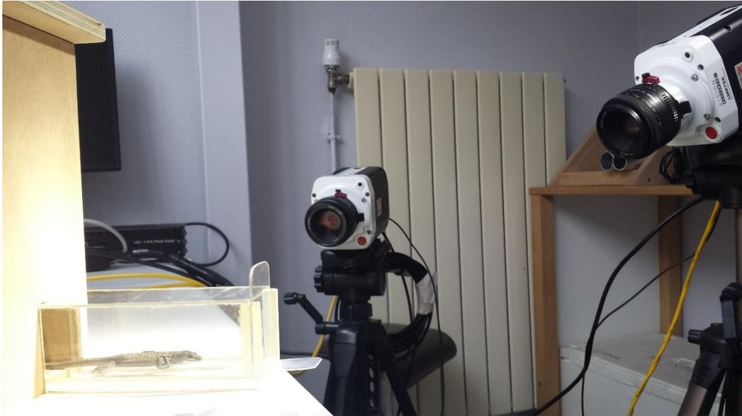
**Figure 1:** Picture of the experimental set-up showing the two high-speed cameras pointing to the end of the tunnel where the prey is positioned. Note the relative position of the cameras which are oriented to form an acute angle allowing to optimize camera calibration and to enhance the accuracy of the three-dimensional tracking.
