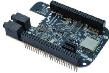
FIGURE 2.12: BeagleBoard Cape - Auxiliary Board
