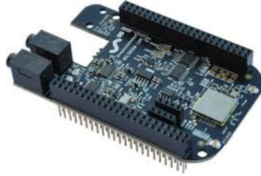
FIGURE 2.12: BeagleBoard Cape - Auxiliary Board
