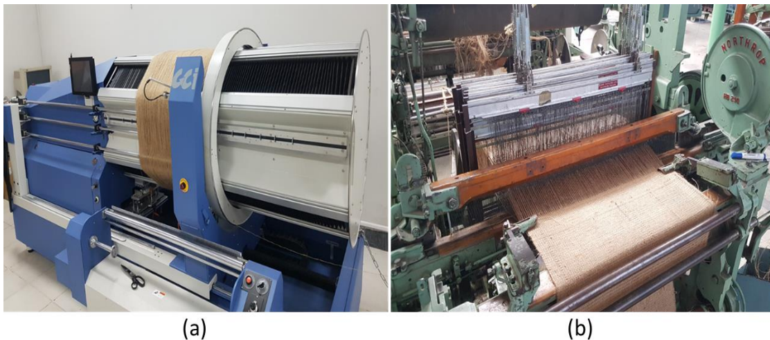
Figure 2.4. (a) Warping and (b) weaving process for 3D jute reinforcement manufacturing
