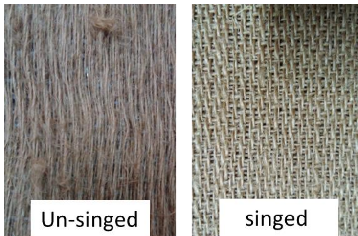
Figure 2.5. The difference in fabric appearance of the un-singed and singed yarn
