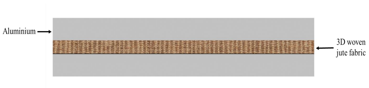
Figure 2.10. 2/1 lay-up configuration used for FMLs fabrication
