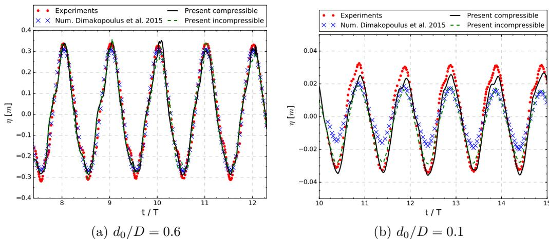
Figure 4.9: In-chamber free-surface elevation averaged over three wave gauges.
