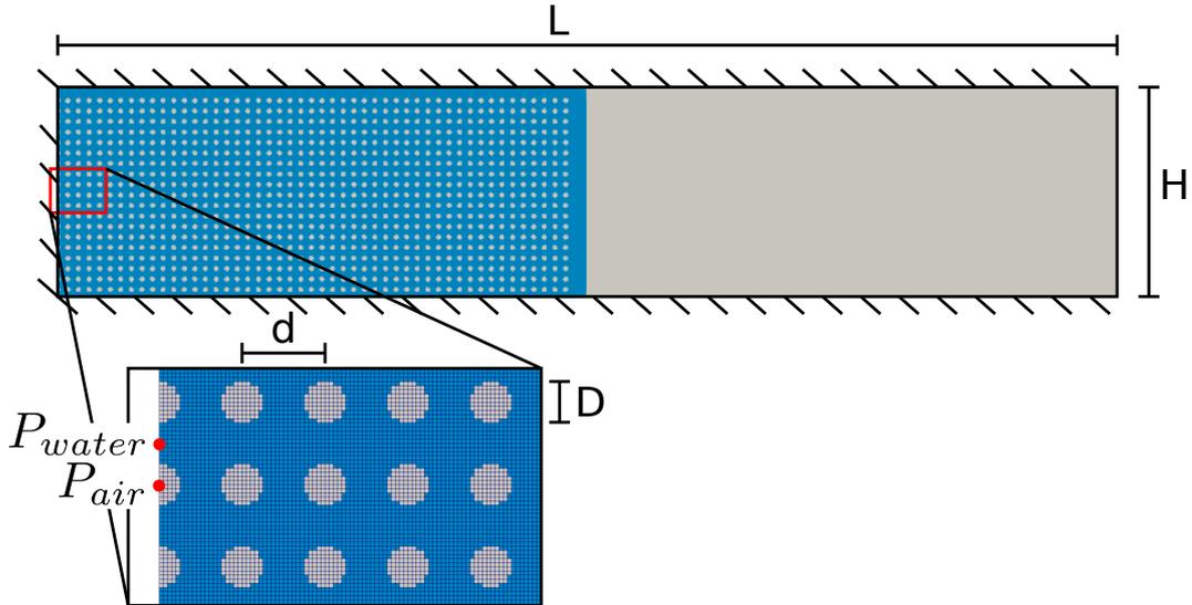
Figure 2.15: Detail of the liquid region initialisation.
