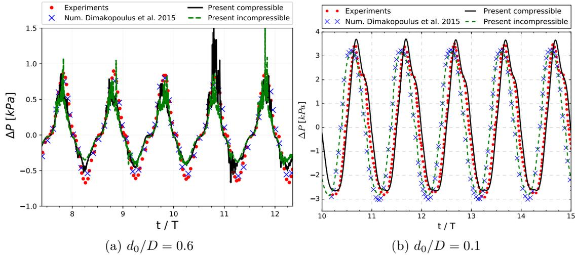
Figure 4.10: Pressure difference across the adjustable orifice.
