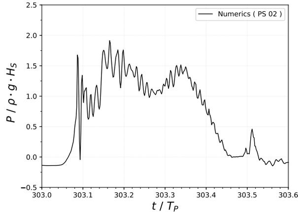
Figure 4.22: Numerical pressure signal recorded by a wall pressure sensor (PS 02) on the exterior front wall during a broken wave impact. Test conditions (Irr11.07):  $H_S = 1m$ ,  $T_P = 6s$  and  $d_0/D = 0.4$ .
