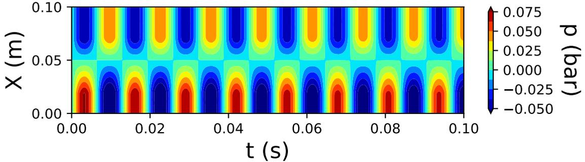
Figure 2.14: Pressure values recorded at the highest and lowest cells compared with the semi-analytic solution using  $\Delta t = 1 \times 10^{-6}$  s.
