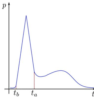
Figure 2.2: Typical pressure record during wave impact
