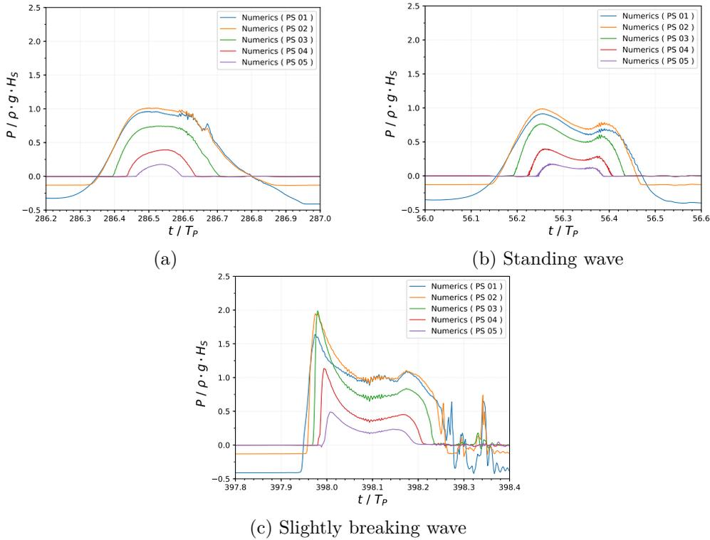
Figure 4.18: Numerical pressure signals recorded by wall pressure sensors (PS 01-05) on the exterior front wall for three distinct characteristic events. Test conditions (Irr11.07):  $H_S = 1m$ ,  $T_P = 6s$  and  $d_0/D = 0.4$ .
