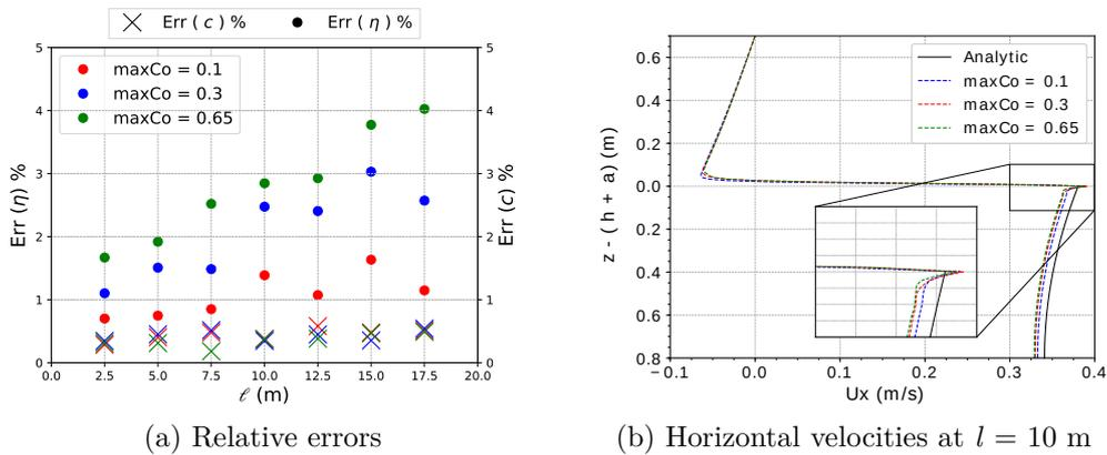
Figure 3.6: Temporal refinement analysis of (left) wave amplitude and celerity relative errors at different distances from the wave maker and (right) horizontal velocities at  $l = 10$  m when  $\eta = \eta_{max}$ . Wave parameters:  $a = 0.1$  m and  $h = 0.7$  m.
