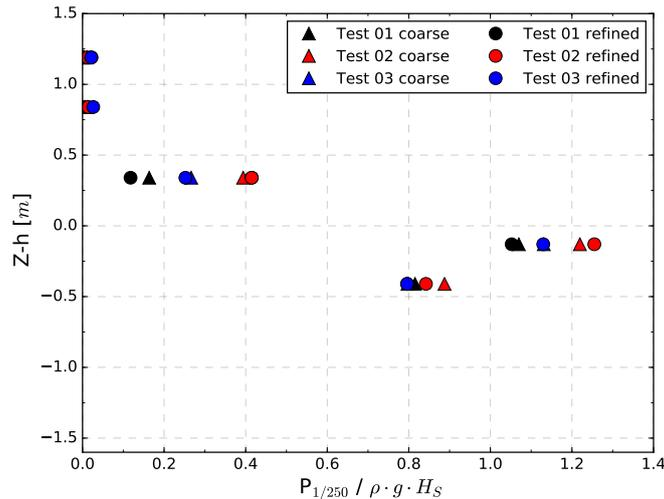
Figure 4.13: Convergence of wave pressure results ( $P_{1/250}$ ) on the structure front wall for 3 exact similar configurations using 3 different wave phase random seeds. Test conditions (Irr01.10):  $H_S = 0.26m$ ,  $T_P = 3s$  and  $d_0/D = 0.6$ .
