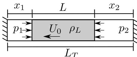
Figure 2.12: 1D liquid piston scheme
