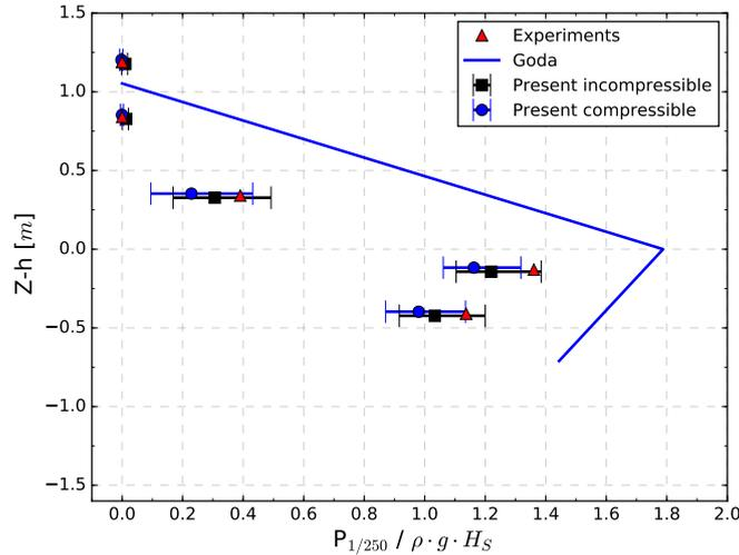
Figure 4.16: Comparison of compressible and incompressible maximal dimensionless wave pressure results ( $P_{1/250}$ ) on the structure front wall evaluated over 5 computation with different phase random seeds. Test conditions (Irr13.01):  $H_S = 0.26m$ ,  $T_P = 4.5s$  and  $d_0/D = 0.4$ .
