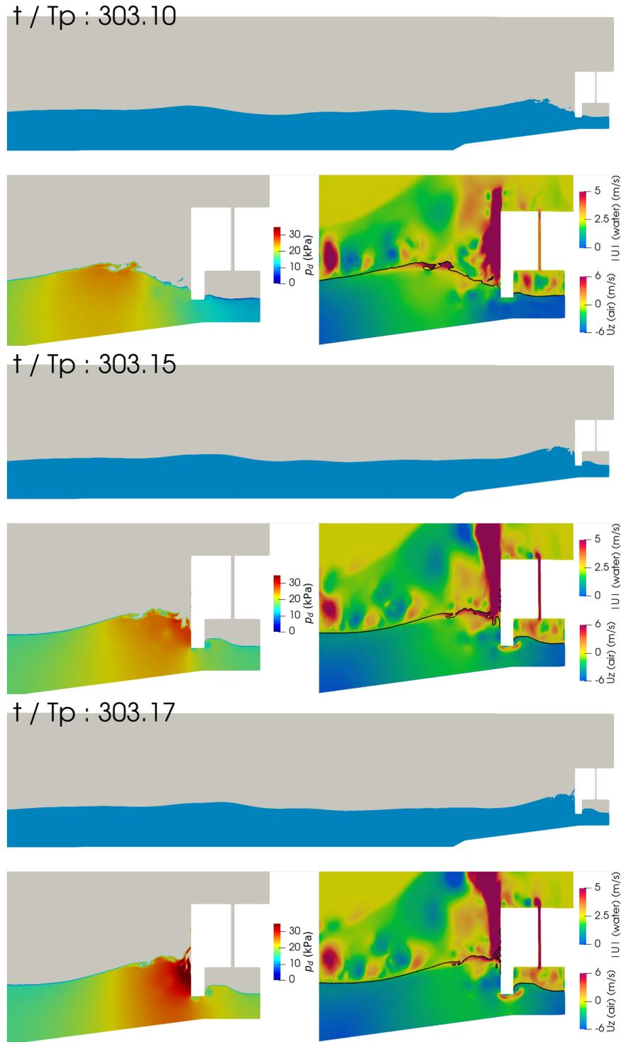
Figure 4.23: Snapshots of (top) water representation  $\alpha > 0.5$ , (bottom left) modified pressure for air  $p_d$  (kPa), (bottom right) velocity magnitude for water  $|U|$  (m/s) and vertical velocity for air  $U_z$  (m/s), for four relevant instants during a broken wave impact, pressure signal Fig. 4.22
