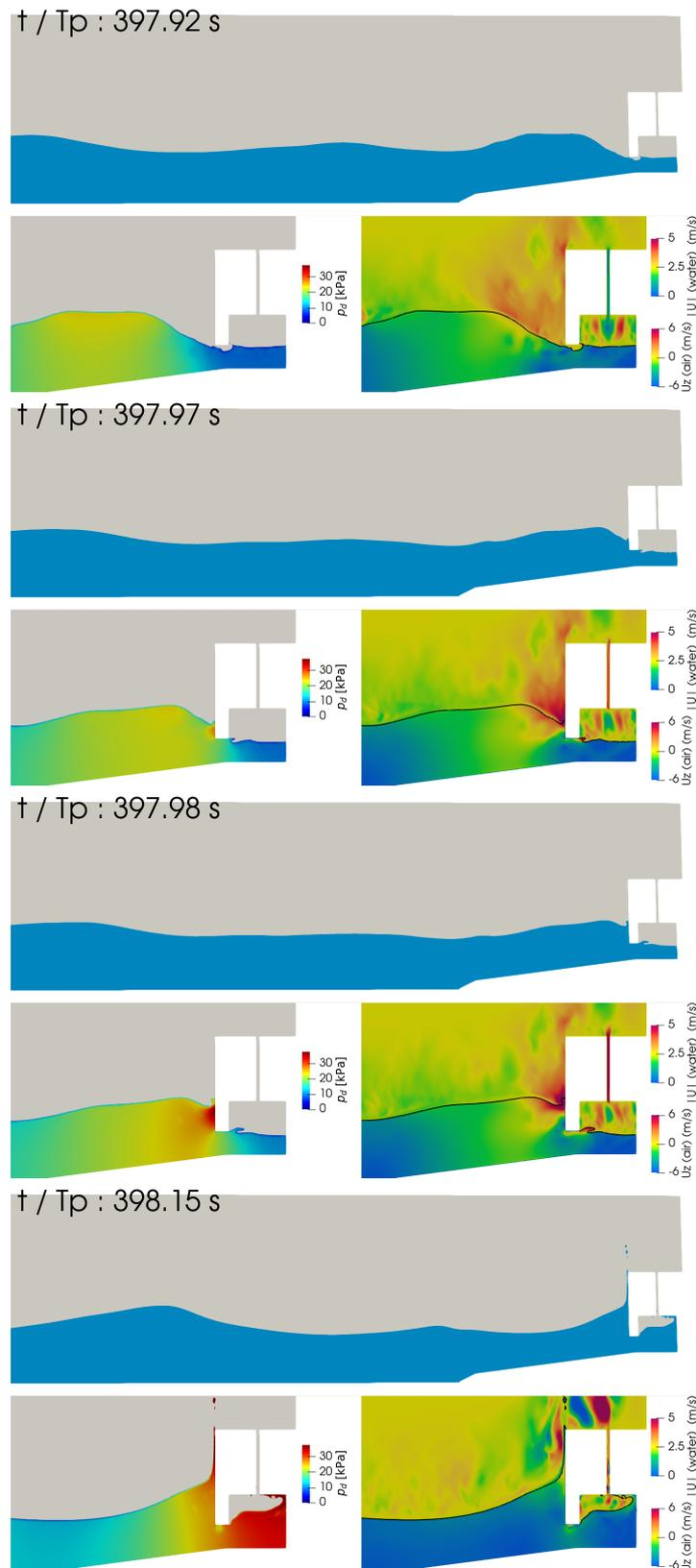
Figure 4.21: Snapshots of (top) water representation  $\alpha > 0.5$ , (bottom left) modified pressure for air  $p_d$  (kPa), (bottom right) velocity magnitude for water  $|U|$  (m/s) and vertical velocity for air  $U_z$  (m/s), for four relevant instants during a wave impact, pressure signal Fig. 4.20
