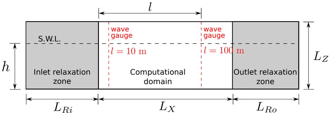
Figure 4.1: Geometrical definition of the numerical wave tank.
