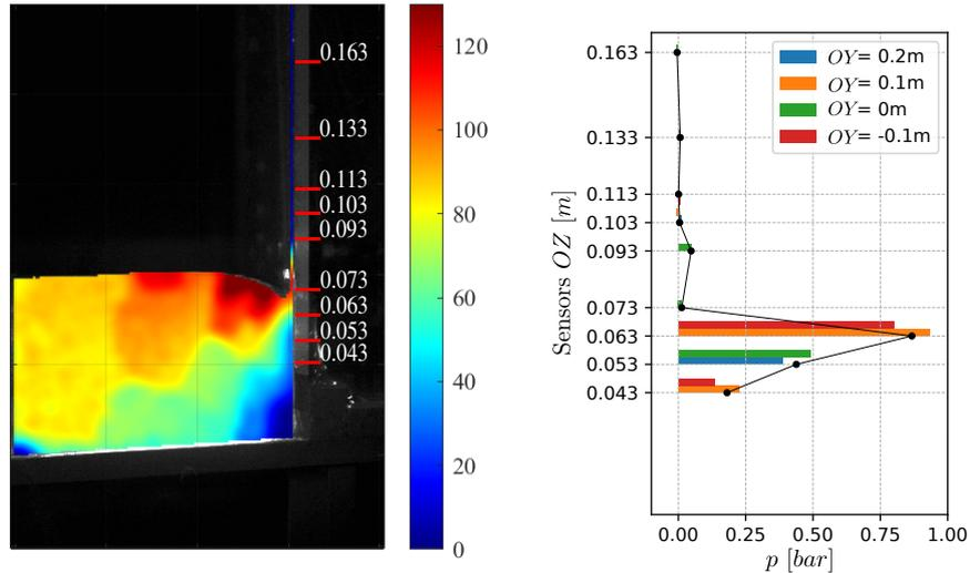
(a) Particle Image Velocimetry of a flip-through impact. Colour range in  $cm/s$
