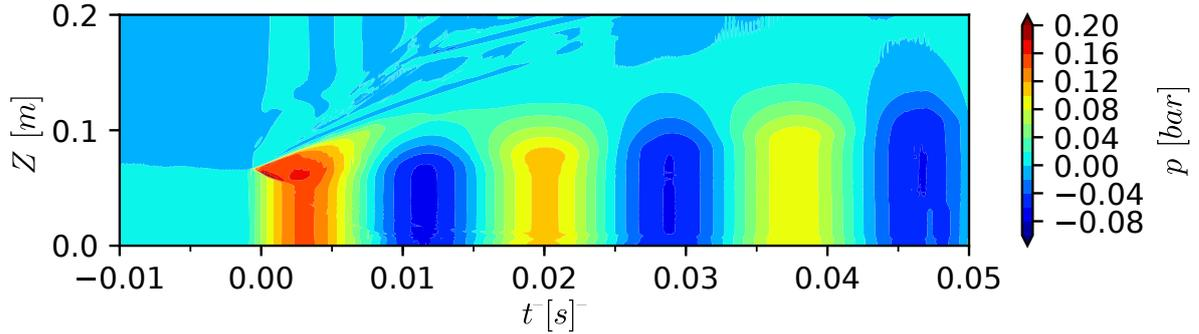
Figure 3.25: Spatio-temporal representation of the wall pressure in the compressible air-pocket impact.
