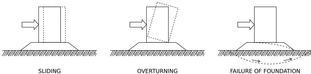
Figure 5: Modes of major failure of vertical breakwater
