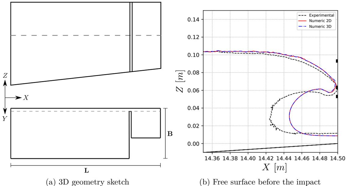
Figure 3.30: 3D air-pocket impact simulation overview
