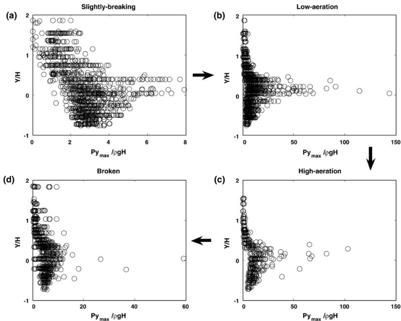
Figure 10: Classification of maximal pressures recorded during the experiments in the GWK by G.N. Bullock *et al.* in 2007 [45]. The pressure values are adimensionalised by the wave height hydrostatic component  $Py_{max}/\rho g H$ , where  $Py_{max}$  is the maximum pressure at each elevation  $y$ . (Note the different horizontal scales)
