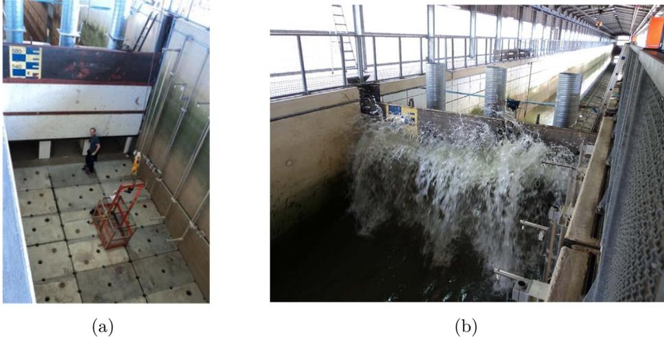
Figure 4.3: Photos from the experimental setup during the installation and the OWC undergoing a wave interaction
