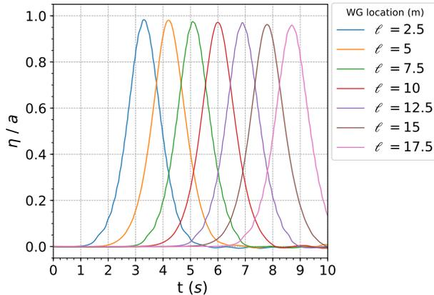
Figure 3.4: Propagation of a Boussinesq solitary wave. Wave parameters:  $a = 0.1$  m and  $h = 0.7$  m.  $l$  corresponds to the wave gauge (WG) distance from the wave maker.
