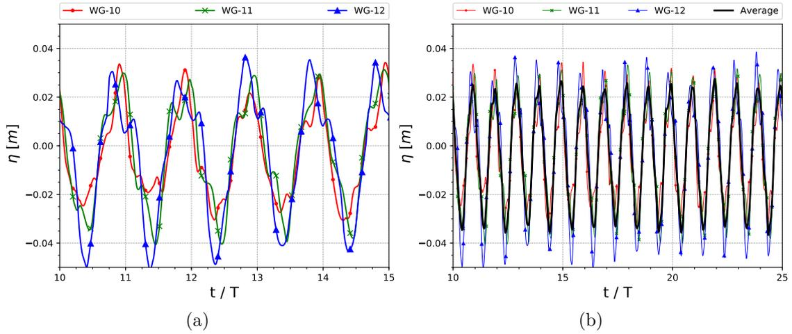
Figure 4.7: Numerical in-chamber free surface elevation averaged over the three wave gauges WG10-WG11-WG12 of Fig. 4.4 issuing from a compressible computation. Test conditions Reg06.10:  $H = 0.4$  m,  $T = 4$  s and  $d_0/D = 0.1$ .
