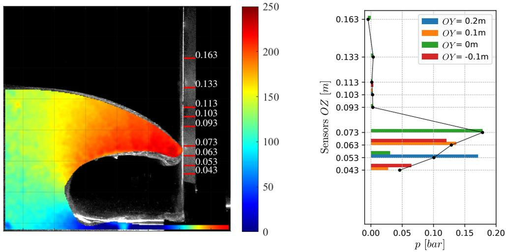
Figure 3.11: Experimental high-aerated or air-pocket impact
