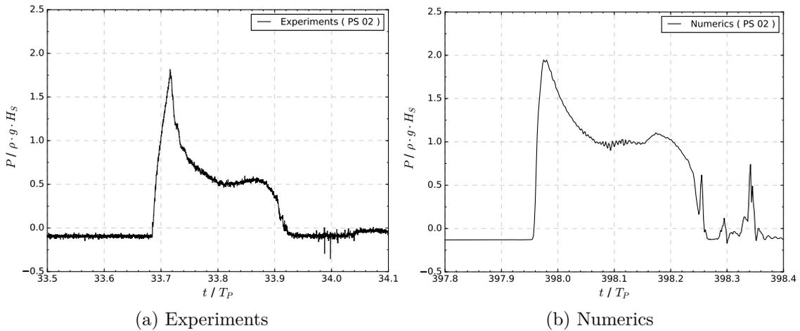
Figure 4.20: Comparison of experimental and numerical pressure signal recorded by wall pressure transducer (PS 02) on the exterior front wall for a violent wave impact. Test conditions (Irr11.07):  $H_S = 1m$ ,  $T_P = 6s$  and  $d_0/D = 0.4$ .
