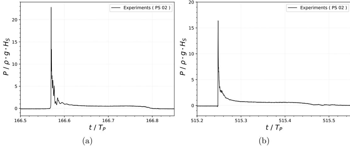
Figure 4.19: Experimental pressure signal recorded by wall pressure transducer (PS 02) on the exterior front wall for two impulsive events. Test conditions (Irr11.07):  $H_S = 1m$ ,  $T_P = 6s$  and  $d_0/D = 0.4$ .
