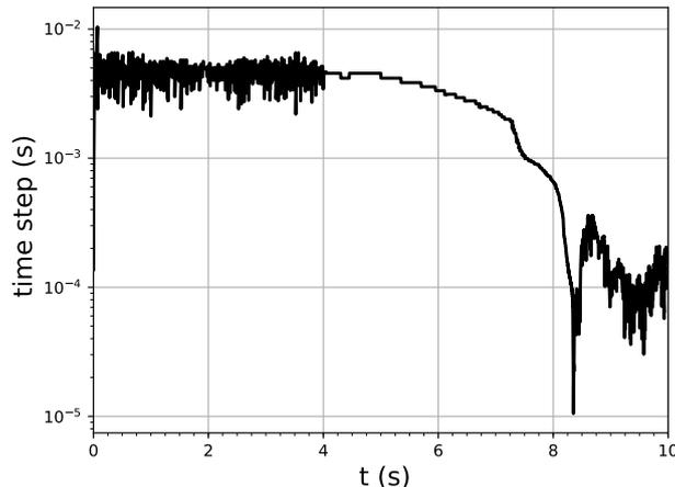
Figure 3.15: Time step evolution during a generation, propagation and an air-pocket impact of a solitary wave in a 2D compressible simulation
