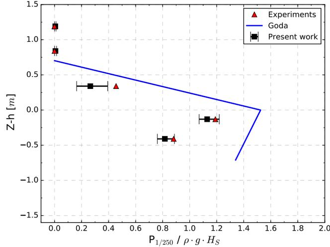
Figure 4.14: Maximal adimensional wave pressure ( $P_{1/250}$ ) ranges over 5 random seeds on the structure front wall compared with the experimental values. Test conditions (Irr01.10):  $H_S = 0.26m$ ,  $T_P = 3s$  and  $d_0/D = 0.4$ .
