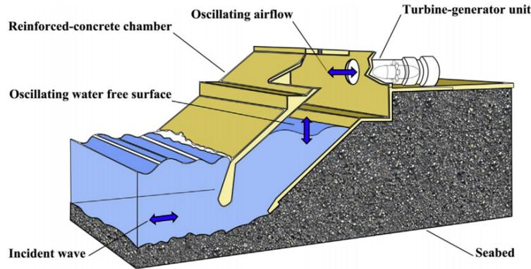
Figure 1: Sketch of an oscillating water column with axial turbine, extracted from [16]
