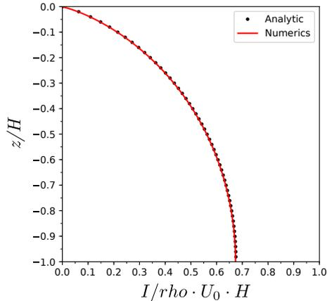
Figure 2.4: Wall pressure impulse distribution compared with the analytic solution,  $\Delta x/H = 2 \times 10^{-3}$  and  $\max\text{Co} = 0.01$ .
