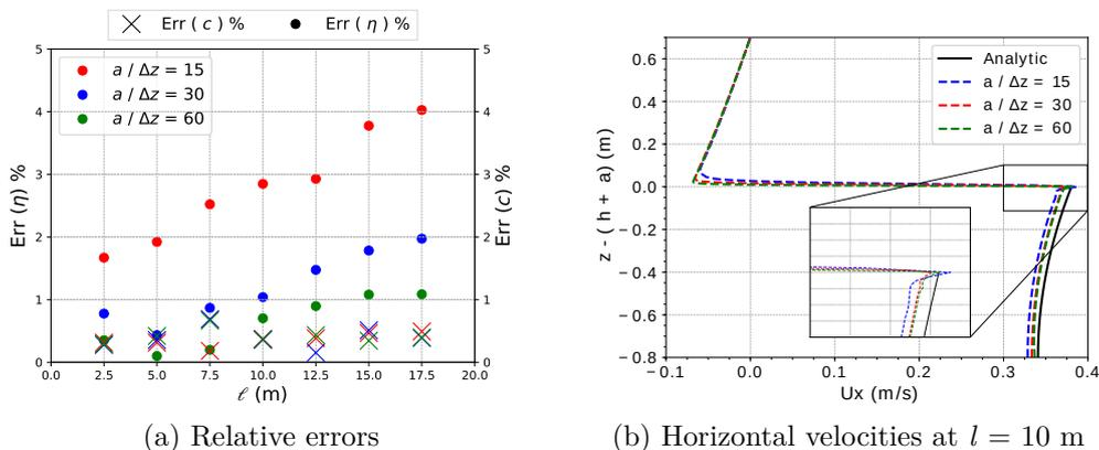
Figure 3.5: Spatial convergence analysis of (left) wave amplitude and celerity relative errors at different distances from the wave maker and (right) horizontal velocities at  $l = 10$  m when  $\eta = \eta_{max}$ . Wave parameters:  $a = 0.1$  m and  $h = 0.7$  m.
