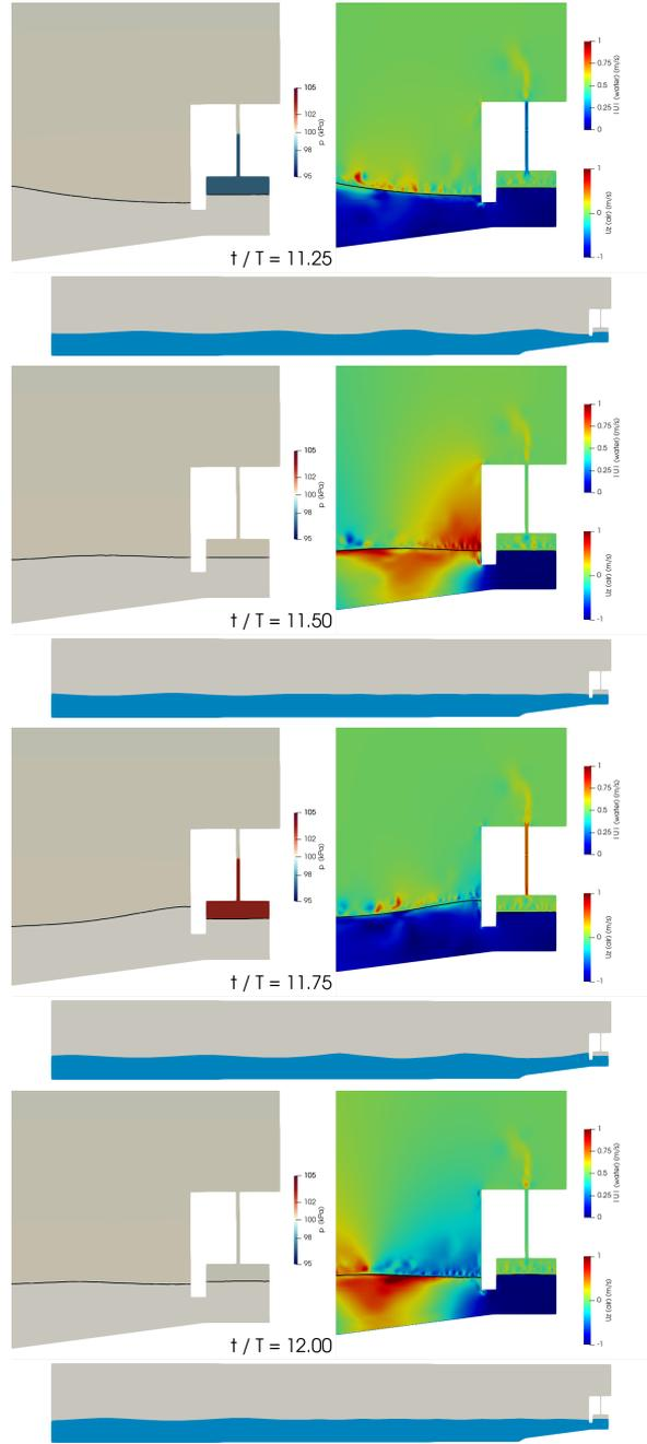
Figure 4.8: Snapshots of an four relevant instants of an OWC undergoing an air-chamber compression and expansion process. Each instant presents (top left) absolute pressure for air  $p$  (kPa), (top right) velocity magnitude for water  $Mag(U)$  (m/s) and vertical velocity for air  $Uz$  (m/s) and (bottom) water representation  $\alpha > 0.5$ .
