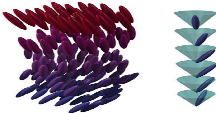
Fig. II.6 – Chiral smectic C phase. The director tilt of each layer precesses upwards around a circle.
