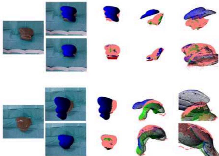
Fig. 6 Results for registration for the two deformations. The initial state of the mesh and the internal markers (in blue) to be registered can be seen in the first row (from three different viewpoints), along with the observed segmented point cloud (pink dots) and the ground truth (the green mesh). The registered meshes are displayed in the second row. For deformation 1, since interactions with the supporting surface are used, we can observe these collisions with the modeled surface (red planes)
