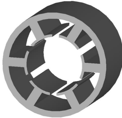
Figure V-1 : Stator 6s4p de la machine Somfy
