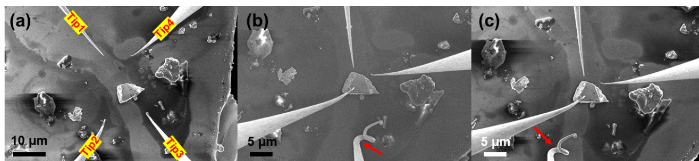
Figure 5.18: (a) Large scale SEM image of an area of the \text{GeCH}_3/\text{Si}(111) sample containing multiple flakes and solvent organic traces. A voltage of -4\text{V} is applied on the four tips. (b) Large scale SEM image of the same area in (a). No voltage is applied on tips 1, 2 and 4. -4\text{V} are applied on tip 3. (c) Large scale SEM image of the same area in (a) and (b). A voltage of -4\text{V} is applied on the four tips. SEM parameters: V=5\text{kV} , I=100\text{pA} .
