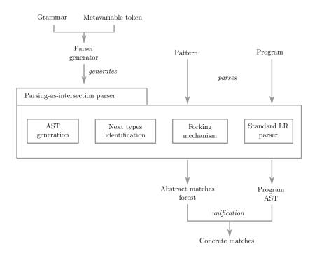
Figure 3.5: General pipeline of the pattern matching engine.
