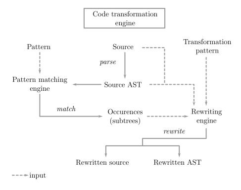
Figure 2.11: Anatomy of a code transformation engine.
