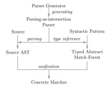
Figure 3.4: Pattern matching engine using parsing as intersection
