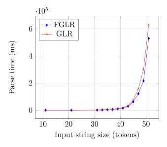
Figure 4.2: FGLR and GLR execution time for highly ambiguous inputs.
