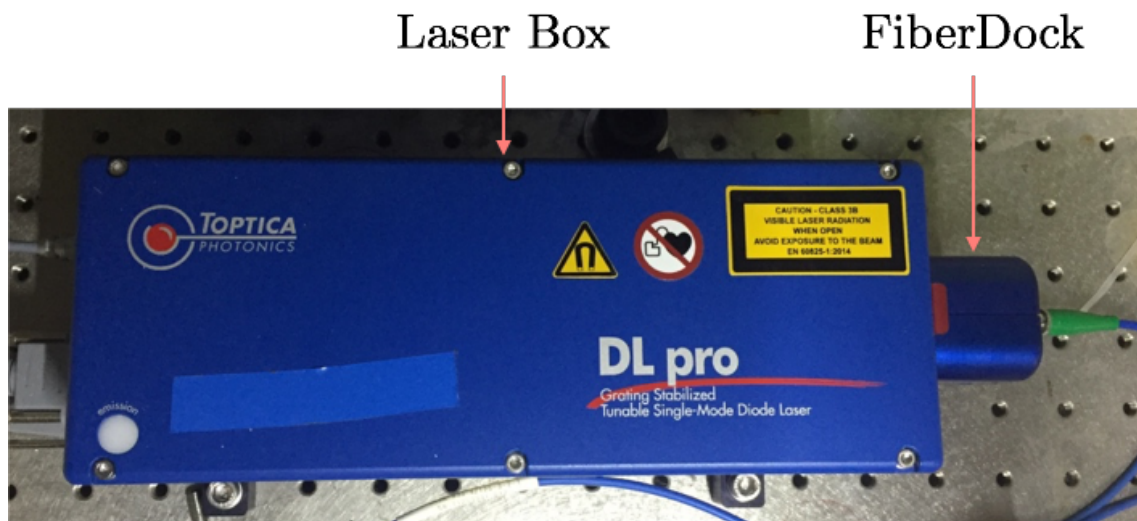
Figure 3.5: Photography of the new Master laser box. The box contains a 670 nm diode laser, an anamorphic prism pair for circular beam shaping and an optical isolator. The FiberDock that is directly connected to the laser box includes an adjustable lens and a fiber coupler. Once the FiberDock is optimized, the power after the fiber is very stable, only requires small adjustments every other week.
