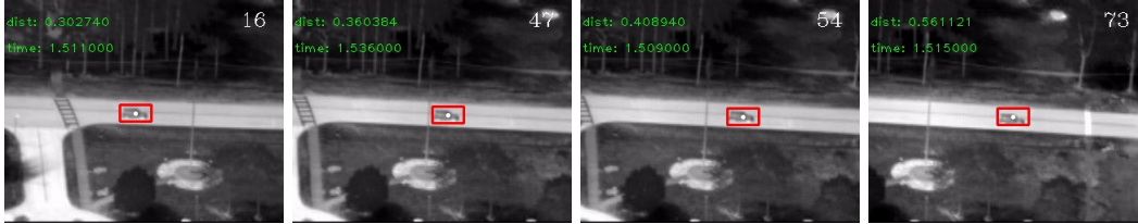
(b) Some detection results using the regularised covariance descriptor on the “Pktest01” sequence.
