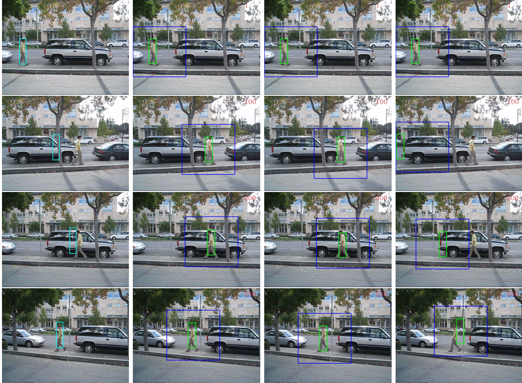
FIGURE 3.7: Tracking results on the “David-outdoor” sequence using different updating policies. Column 1: “MILTracker”. Column 2: “AdpCov+cu”. Column 3: “AdpCov+nu”. Column 4: “AdpCov+fu”. In the last three columns, the blue rectangles indicate the search windows and the green rectangles show the tracking results. Row1: frame #1. Row 2: frame #100. Row3: frame #200. Row4: frame #250.
