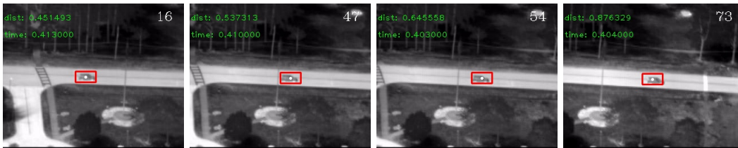
(c) Some detection results using the adaptive covariance descriptor on the “Pktest01” sequence.
