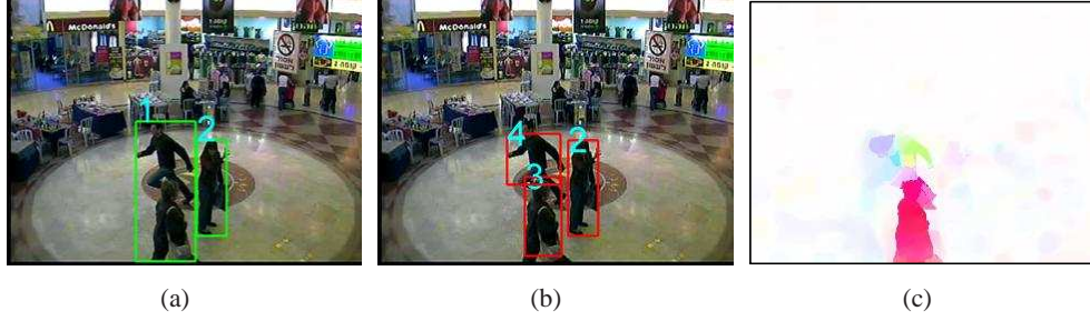
Figure 3.9: The blobs of the objects before and after our proposed blob extraction method. (a) 2 extracted blobs based on the foreground template. (b) 3 extracted blobs via the proposed blob extraction method, which is based on the foreground template and the optical flow. (c) The optical flow image of Fig.(a)(b). A black border is added to illustrate the image clearly.
