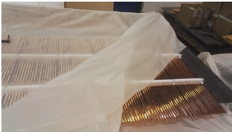
Figure 2.16: One of the coil panel, recycled from NEMO-3.
