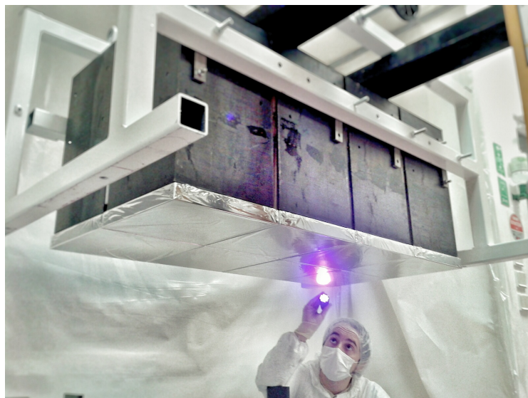
Figure 2.17: A block of 8 optical modules grouped together for installation at LSM. The magnetic shields are the black boxes surrounding the optical modules.
