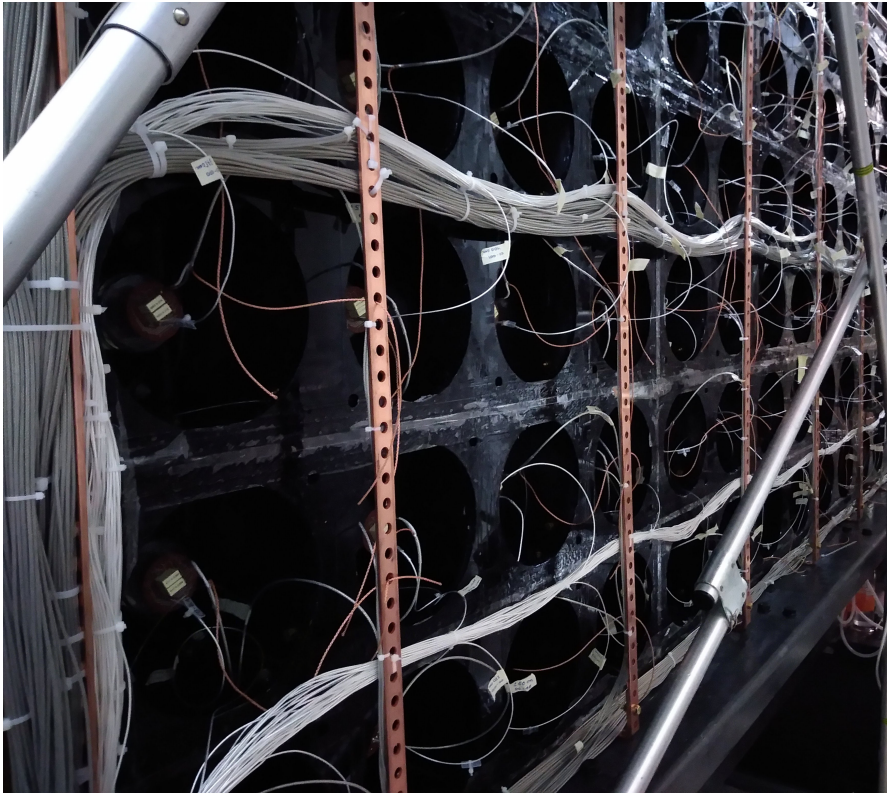
Figure 2.21: Back view of one main calorimeter wall. Signal cables are white and thin, HV cables are grey and thick.
