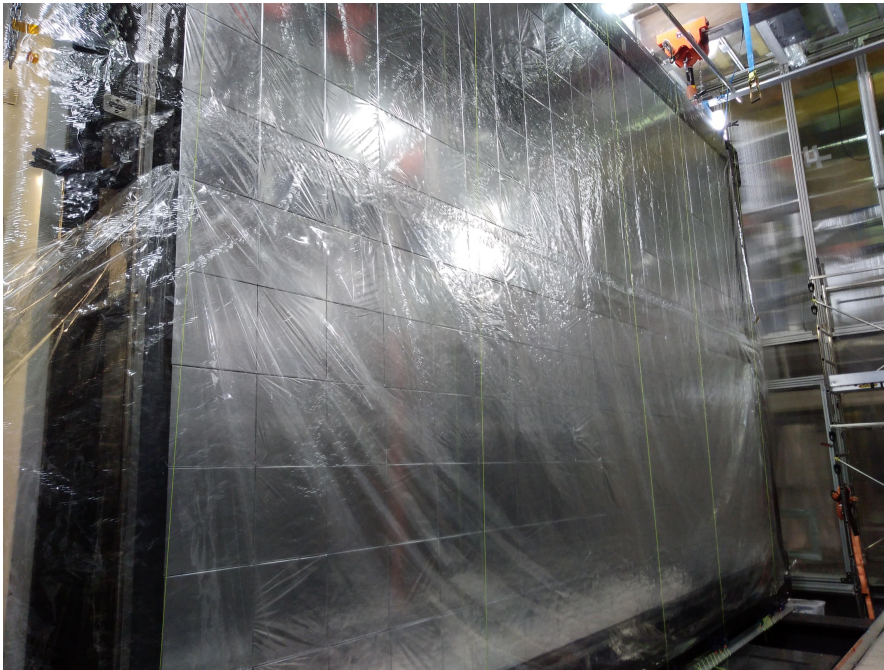
Figure 2.25: Piece of radio-pure nylon film installed on the front face of each calorimeter main walls.
