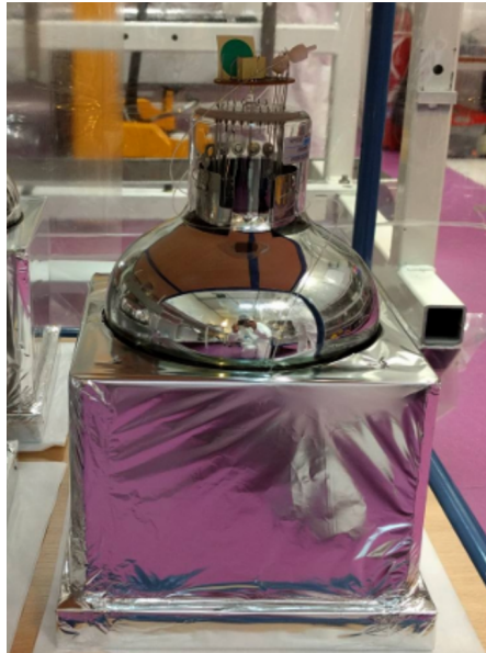
Figure 2.11: A scintillator coupled with a PM. The shiny wrapping around the scintillator is the aluminised Mylar.
