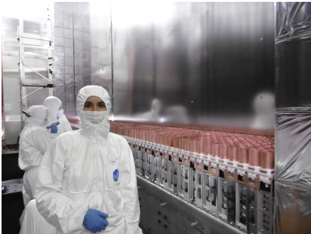
Figure 2.7: Inside view of the tracker (with me standing in the foreground), before detector closing, on the day of the wire check, looking for possible broken wires at the base of the copper rings.
