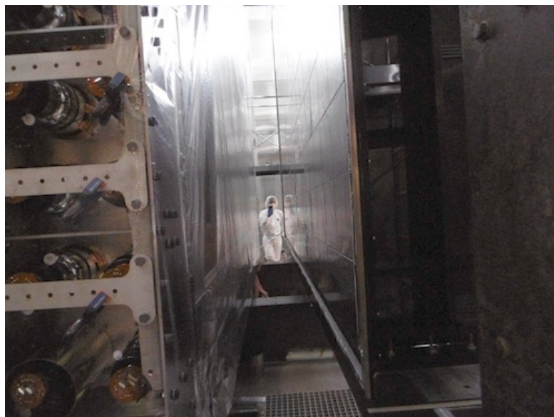
Figure 2.1: Last picture of the SuperNEMO demonstrator before closing it, the 22 November 2018. The picture is taken from one side of the detector, facing the other side. We can distinguish on the right the front of one of the two calorimeter main walls, and on the left one of the two tracker chambers.
