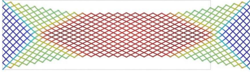
Figure 3: The three different deformation zones in the pantographic structure during an extension test: no deformation (blue), shear at macro level and relative rotation at micro level (red) and shear with a different angle (green). The bending of fibers is concentrated in the interface zones.
