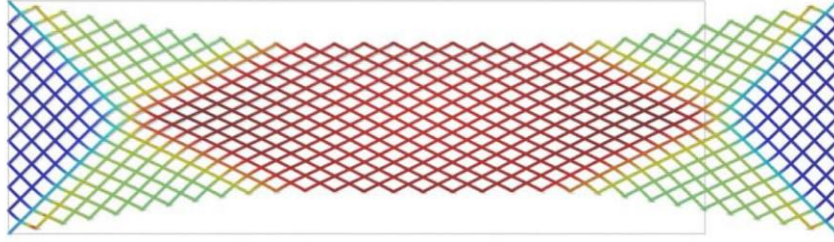
Figure 1.21: The three different deformation zones in the pantographic structure during an extension test: no deformation (blue), shear at macro level and relative rotation at micro level (red) and shear with a different angle (green). The bending of fibers is concentrated in the interface zones.
