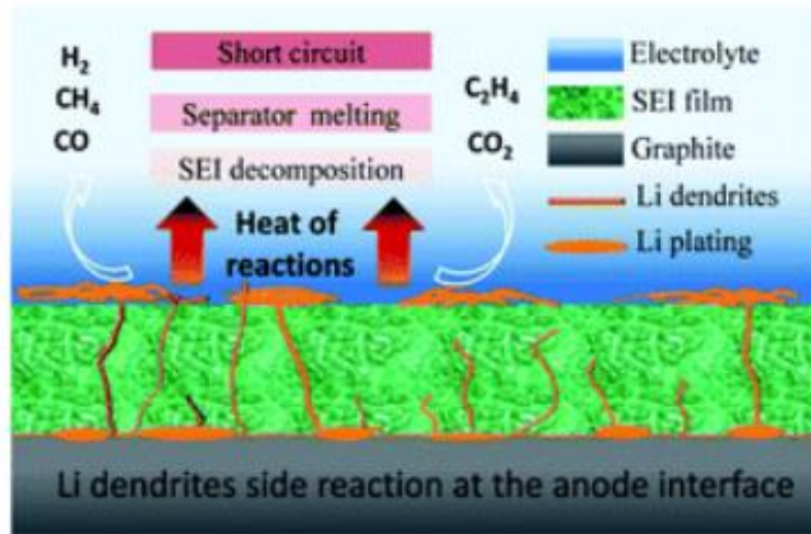
Figure 18: Scheme of phenomena responsible for LIBs failure. 35
