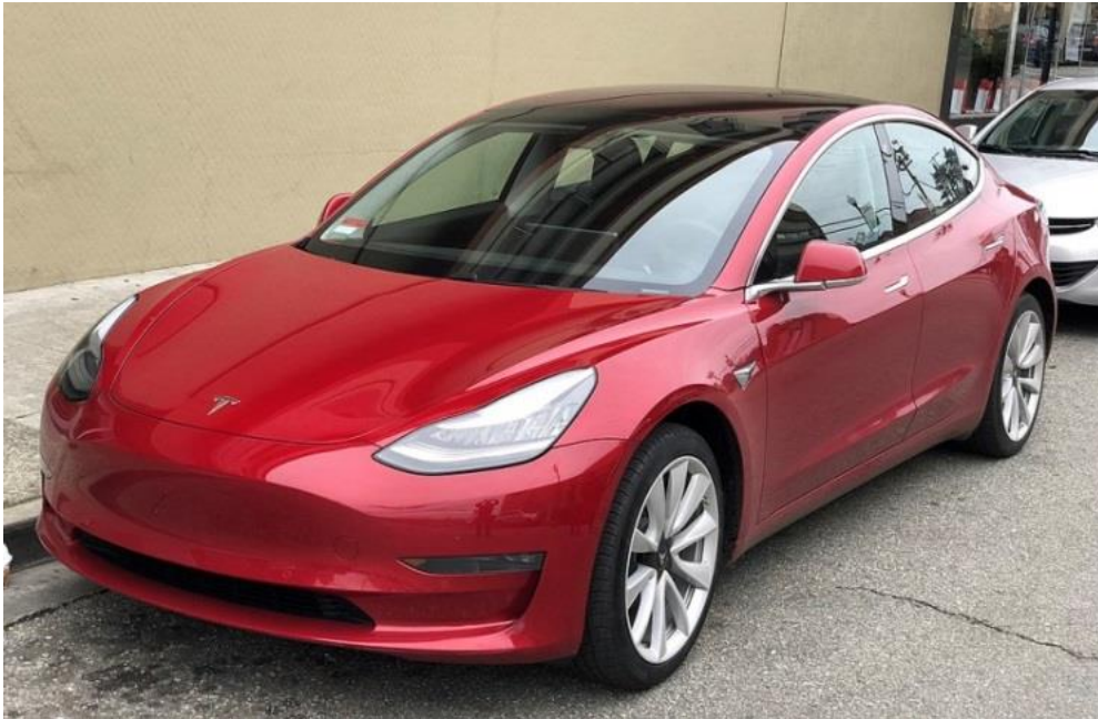
Figure 12: Tesla “Model 3”, a fully- electric four-door automobile with a range of 345 km at a cost of 35000 US$ (2017). 22
