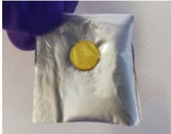
Figure 67: Ar-filled coffee bag with kapton foil window, used to analyze the SS disc after cycling.
