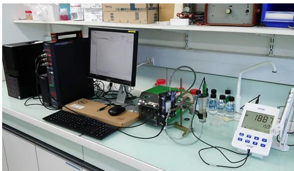
Fig 3.12 Picture of laboratory setup of CDI experiment.
