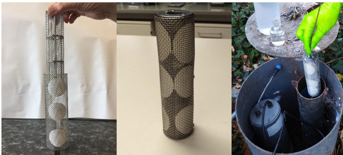
Figure S1. Photographs of ED supports designed specially adapted to GW well dimensions.
