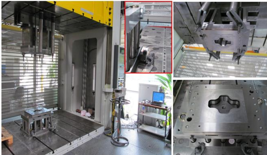
Fig. 3-35. Experimental setup for cross-section deep drawing tests (IUL/TUD).
