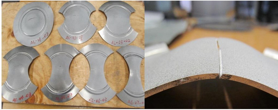
Fig. 3-32. Post-mortem of NAK after loading (IUL/TUD).
