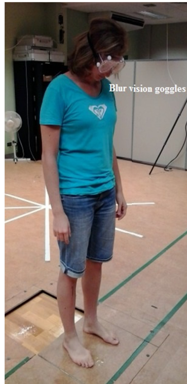
FIGURE 20: ILLUSTRATION OF THE BLUR GOGGLES FOR VISUAL ACUITY DEGRADATION.
