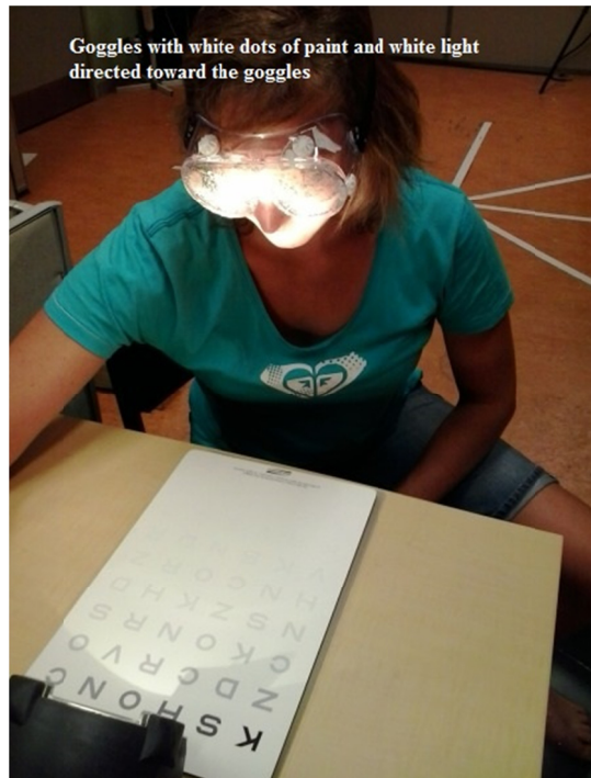
FIGURE 21: ILLUSTRATION OF THE CONTRAST DEGRADATION GOGGLES.
