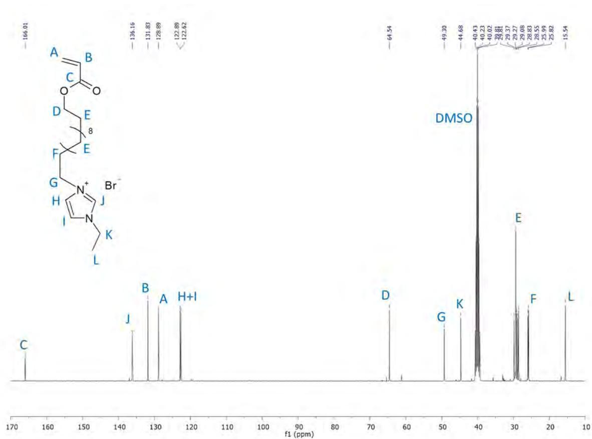
FIGURE C.30 – <sup>13</sup>C-NMR of ADEIBr in DMSO-d<sub>6</sub> at 298 K.
