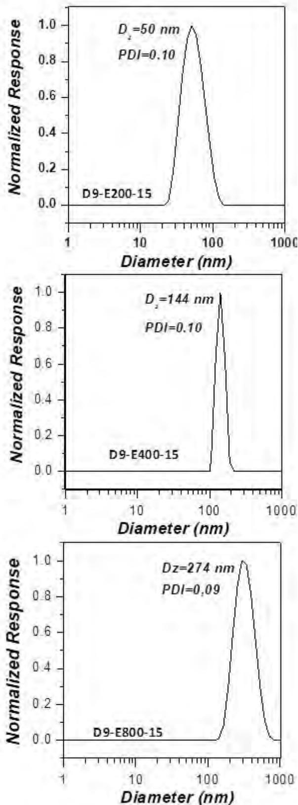
FIGURE C.41 – DLS in water of D<sub>9</sub>-E<sub>200</sub>-15, D<sub>9</sub>-E<sub>400</sub>-15 and D<sub>9</sub>-E<sub>800</sub>-15.
