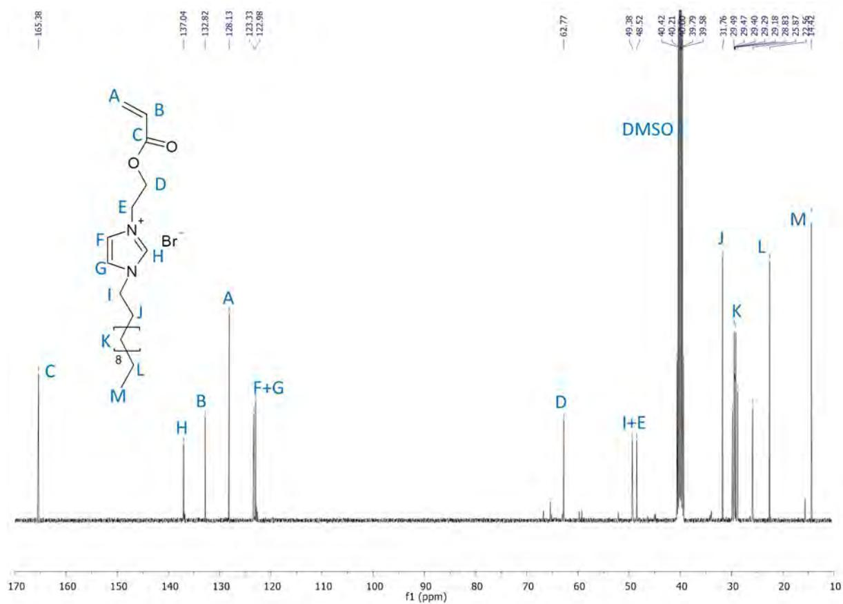
FIGURE C.33 –  $^{13}\text{C}$ -NMR of AEDIBr in  $\text{DMSO-d}_6$  at 298 K.
