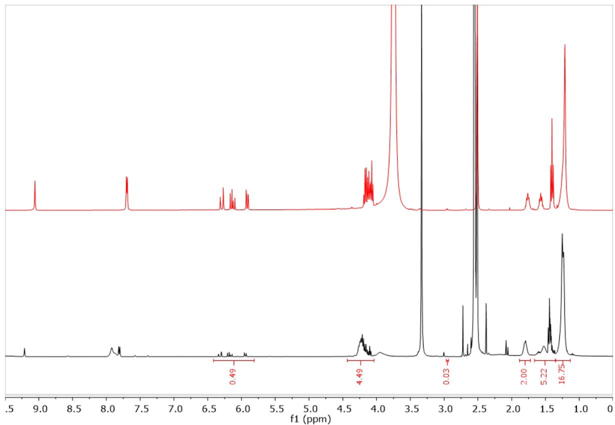
**FIGURE C.36** – <sup>1</sup>H NMR of ADEIBr polymerization medium (in DMSO-d<sup>6</sup> at 298 K), using EMP as a CTA and ACPA as an initiator ([ADEIBr] : [EMP] : [ACPA] = 100 : 1 : 0.2) at t<sub>0</sub> (a) and t<sub>f</sub> (83 % of conversion) (b).
