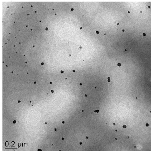
**FIGURE C.40** – Representative TEM picture of PIL block copolymer spherical nanoparticles obtained at 5 wt% solid contents (D<sub>9</sub>-E<sub>600</sub>-5).
