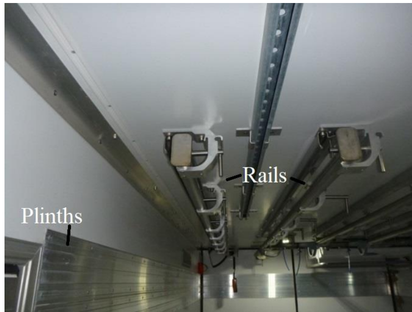
Figure 2.23 Meat rails and plinths inside of a refrigerated vehicle.
