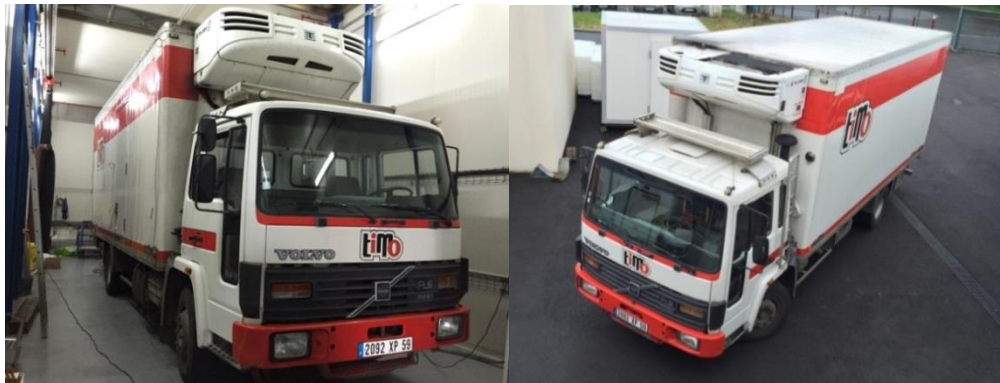
Figure 2.49 Insulated enclosure built with a double panel system. 30 years old French refrigerated truck in Cemafruid ATP test laboratory in 2016.
