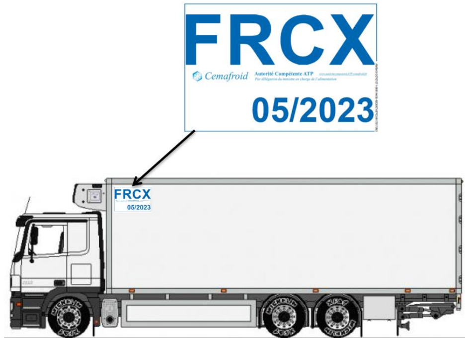
Figure 2.37 Correct application of the ATP identification mark.
