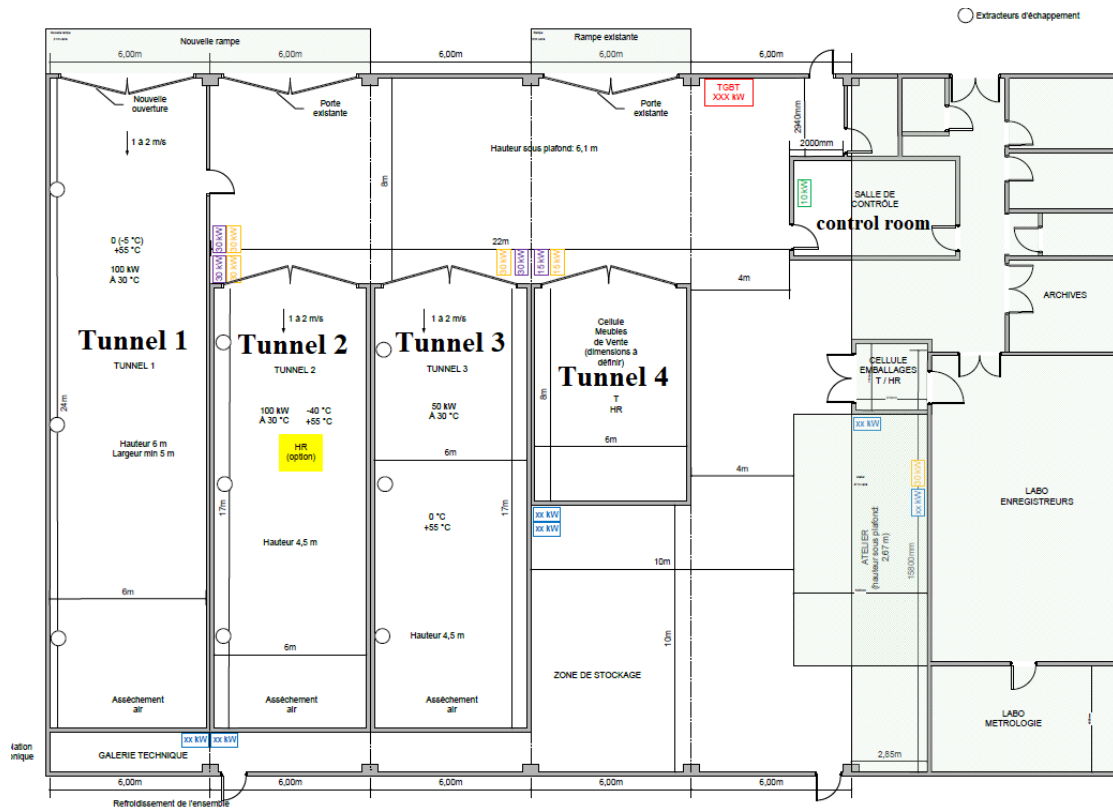
Figure 3.1 Plan of the climatic chambers in Cemafruid.
