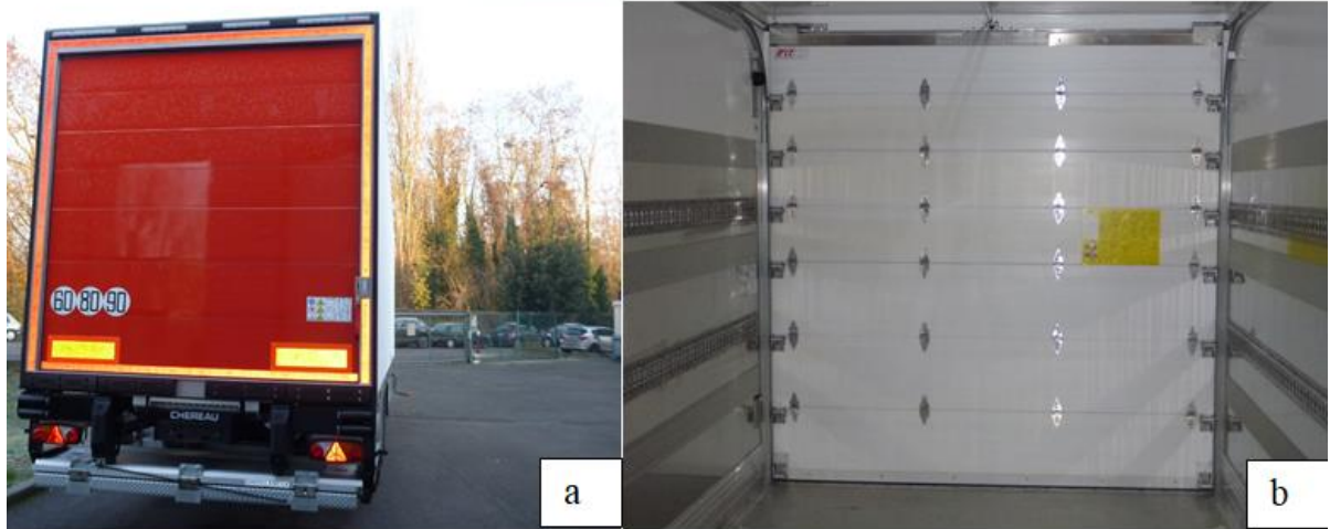
Figure 2.26 Sling shutter door : a) view from the outside; b) view from the inside.
