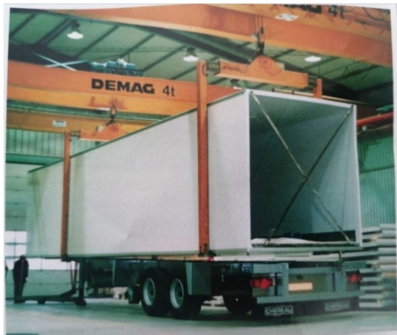
Figure 2.48 Anchoring of the insulated enclosure on the frame of the vehicle (Cadet, 2004).
