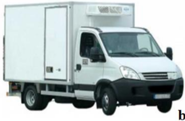
Figure 1.6 a) Integrated insulated vehicle; b) Reported insulated vehicle.
