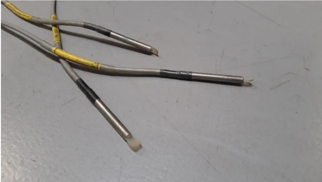
Figure 3.8 Four wire platinum resistance thermometers type Pt100 used in Cemafruid.
