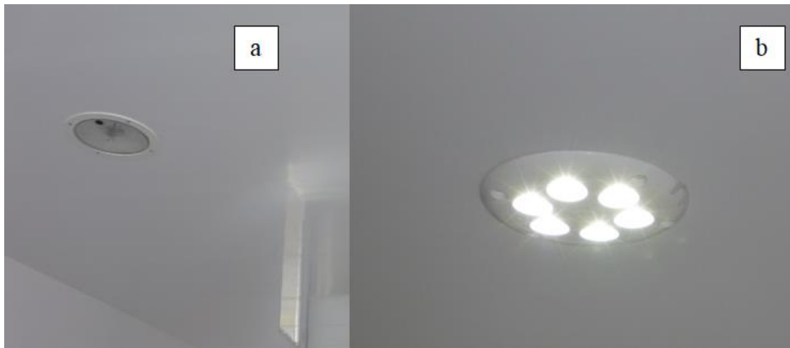
Figure 2.25 Example of lightings inside of a refrigerated vehicle: a) recessed lighting; b) surface lighting
