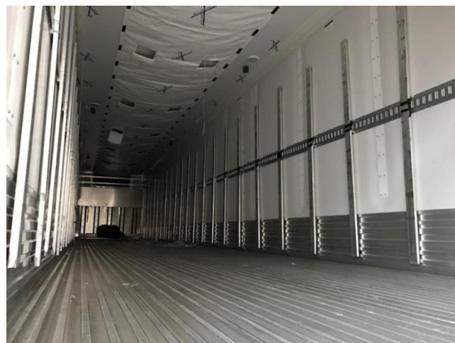
Figure 2.19 Interior view of a refrigerated container showing ‘T’ bar floor.
