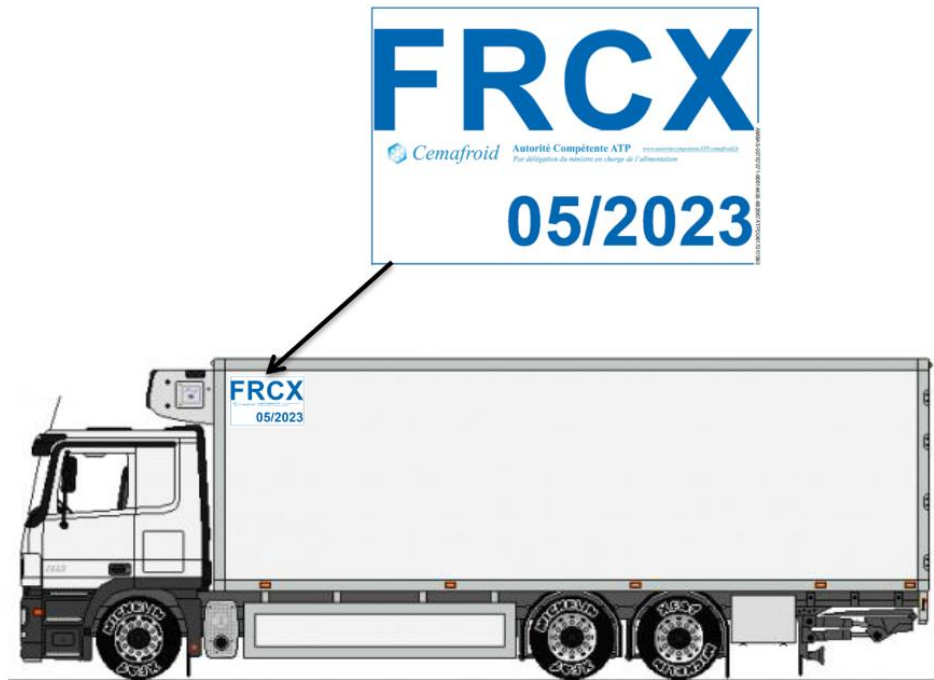
Figure 2.37 Correct application of the ATP identification mark.
