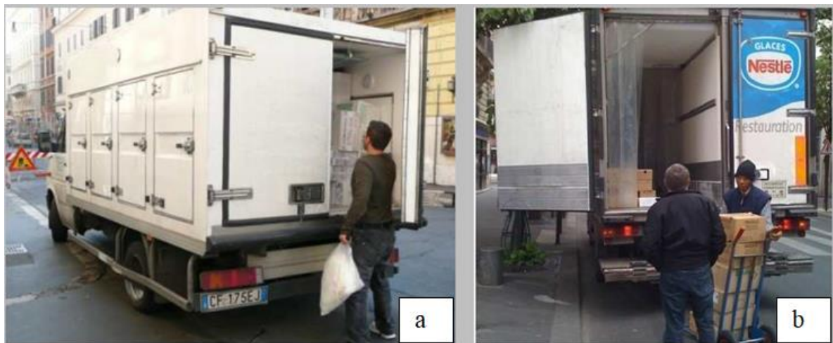
Figure 2.27 Total rear opening with two leaves a) without plastic curtains; b) with plastic strip curtains. (Cavalier, 2010).
