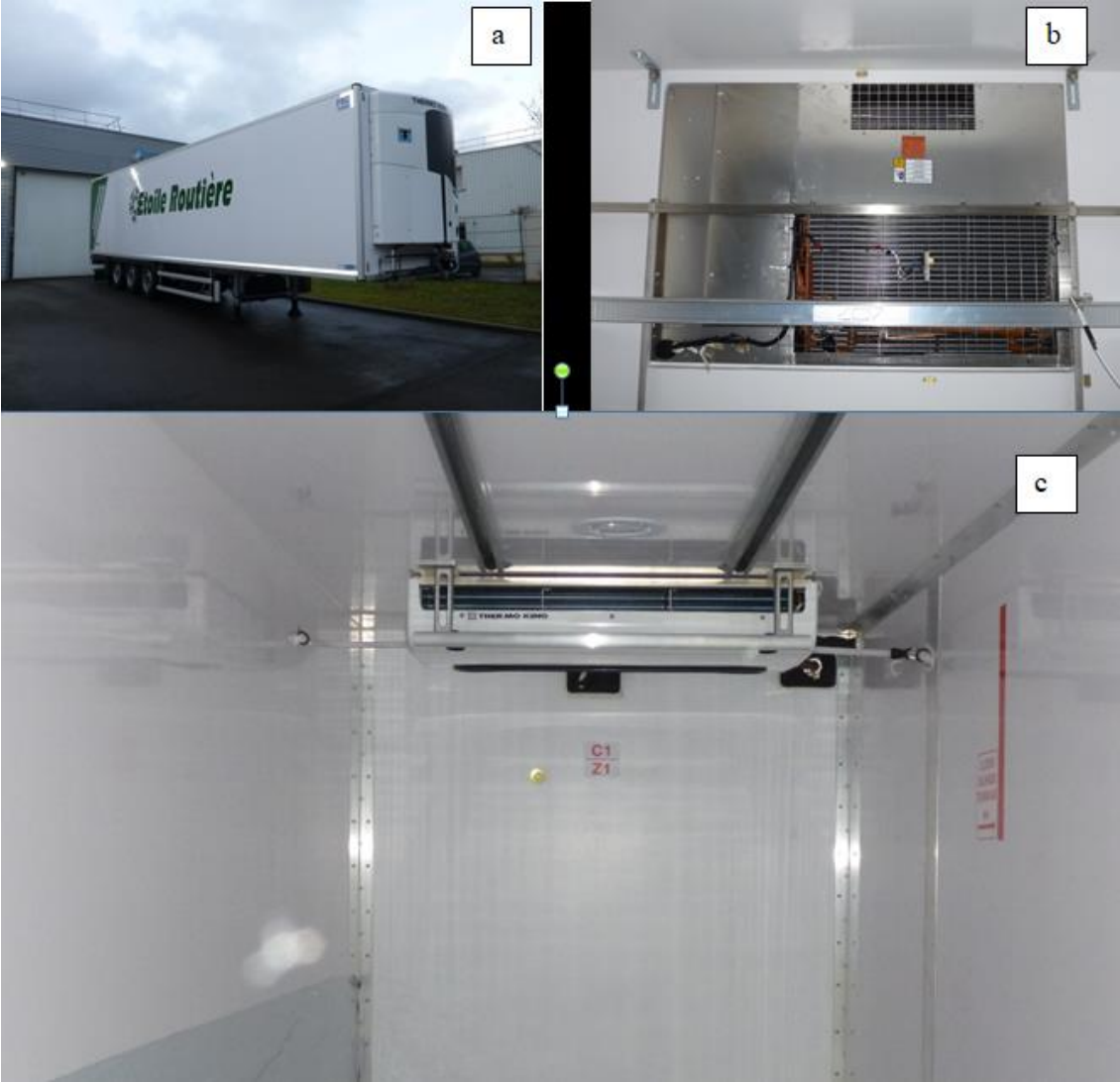
Figure 2.18 a) Monobloc architecture of a refrigerating unit, view from the outside; b) monobloc architecture of a refrigerating unit, view from the inside; c) split architecture of a refrigerating unit, view from inside.
