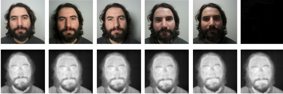
Figure 2.5: Impact of illumination variation on the visible and the thermal spectrum.
