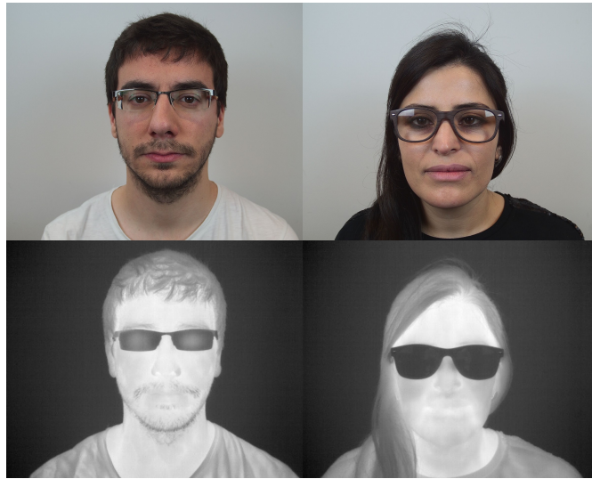
Figure 2.6: Impact of eyeglasses on the visible and the thermal spectrum.
