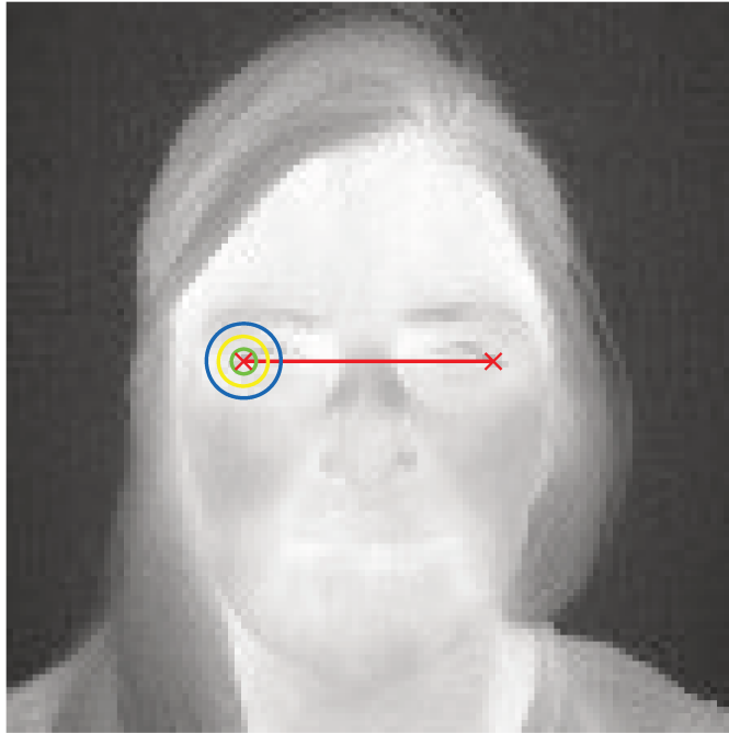
Figure 6.3: Inter-ocular distance (IOD) marked in red and circles denoting different detection error thresholds, green: 0.05, yellow: 0.1, blue: 0.15 times IOD.
