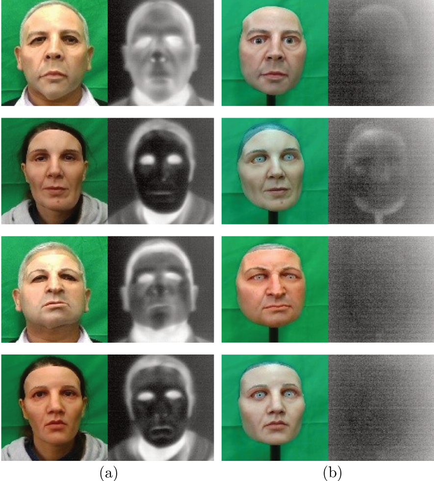
Figure 7.4: Samples of presentation attack of CSMAD database in visible and thermal spectrum. (a) worn masks (b) standing masks.
