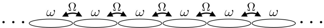
FIGURE D.1: Nanowires chain. Each wire resonate at \omega and the coupling factor between two wires is \Omega .
