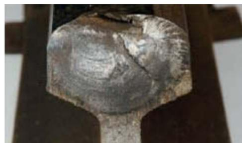
Figure 2.15: Gauge corner cracking [112]
