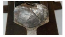
Figure 2.14: Rail head checking [98]
