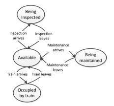
Figure 8.3: Track component working status model
