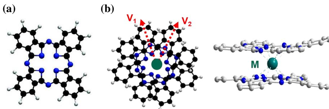
**Fig. 3.1:** (a) Model of phthalocyanine ligand (Pc), the chemical formula is  $\text{C}_{32}\text{H}_{18}\text{N}_8$ . Color code: Blue = Nitrogen; Black = Carbon; White = Hydrogen; Green =  $\text{M}$  (Terbium or Yttrium). (b)  $\text{MPc}_2$  molecule, Top and side view,  $V_1$  and  $V_2$  are respectively the symmetry axis of the upper and lower Pc.
