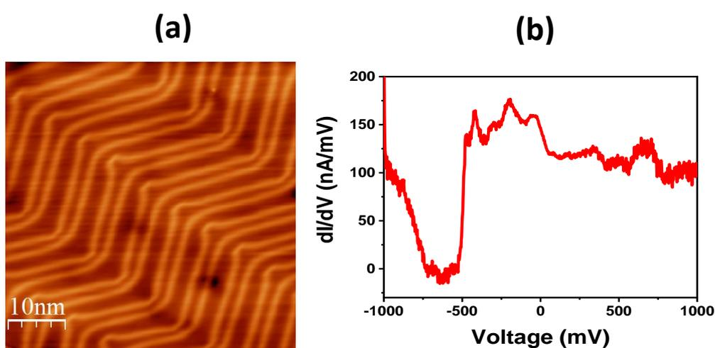
**Fig. 2.5:** Example of experimental results obtained by STM / STS on an Au(111) surface. (a) Topographic STM image showing surface reconstruction. (b) conductance spectrum revealing Shockley state (-500 mV) as a step.
