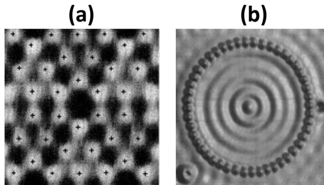
**Fig. 2.6:** (a) Reconstruction ( $7 \times 7$ ) of a surface of Si(111), taken from [3]. (b) Spatial image of the eigen states of a quantum corral formed by manipulation of 48 Fe atoms on Cu(111), taken from [2].
