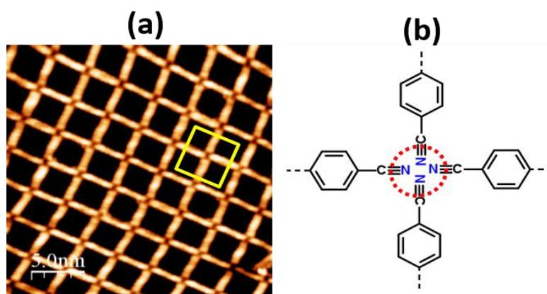
**Fig. 5.5:** (a) High – resolution STM image showing a square lattice of NC-Ph<sub>5</sub>-CN linkers. (b) Yellow square in (a), corresponding schematic model showing the interaction (dashed red line) between adjacent carbonitriles endgroup.
