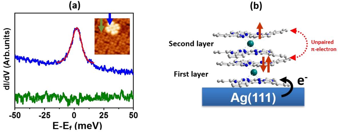
**Fig. 4.6:** (a)  $dI/dV$  spectra showing a Kondo resonance (blue line) on the ligand of the molecule in second layer, the peak disappears when the tip is positioned above first layer. (b) Basic schematics of  $(TbPc_2)_2$  (first and second layer) show: The pairing of two electrons in the first layer caused by charge of the  $Ag(111)$  substrate, and the appearance of the delocalized electron in molecule of second layer resulting the Kondo resonance.
