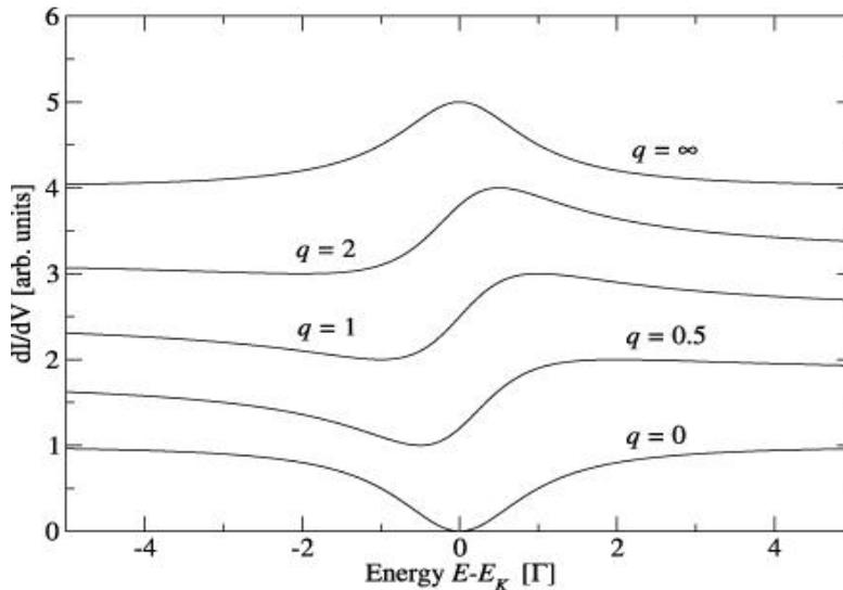
**Fig. 1.11:** Set of curves calculated with the normalized Fano equation for different  $q$  values [45]. At  $q = 0$  a Lorentzian dip is detected which corresponds to mainly direct tunneling. In the limit of large  $q$ , a Lorentzian peak is formed corresponding to mainly indirect tunneling. Intermediate values of  $q$  result in an s-like curve.
