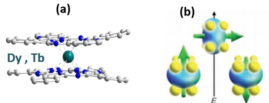
**Fig. 1.4:** (a) Sandwich-type crystal field for LnPc<sub>2</sub> single-molecule magnet design. (b) Depictions of low- and high-energy configurations of the f-orbital electron density with respect to the crystal field environment for a 4f ion of oblate electron density. The green arrow represents the orientation of the spin angular momentum coupled to the orbital moment. reproduced from [17].
