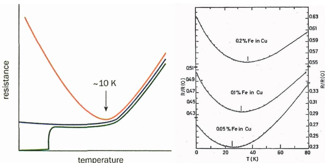
**Fig. 1.6:** (a) Qualitative variation of the resistivity of a metal with temperature. Normal metal (blue), superconducting metal (green), diluted magnetic alloy (red) (extract of [41]). (b) The minimum resistance as a function of temperature for the copper (Cu) crystal with different concentration of iron (Fe) impurities.
