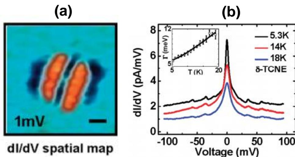
**Fig. 1.13:** (a)  $dI/dV$  Mapping of the density of state near Fermi level for a TCNE molecule showing the localization of Kondo resonance. (b)  $dI/dV$  spectroscopy near Fermi level on a TCNE molecule deposited on Cu(111) showing Kondo resonance at different temperatures (5.3 K, 14 K and 18 K). (Extracted from [52])
