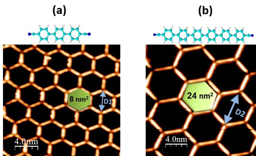
**Fig. 5.11:** (a) and (b) High-resolution STM image of the honeycomb networks of Co(NC-Ph<sub>3</sub>-CN)<sub>3</sub> and Co(NC-Ph<sub>6</sub>-CN)<sub>3</sub> respectively, showing the diameters (cyan area) and (green area) of porous nanomeshes of the two networks.
