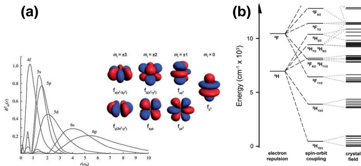
**Fig. 1.2:** (a) Radial distribution functions of 4f, 5s, 5p, 5d, 6s and 6p electrons for cerium [12]. *Inset* The 4f orbitals from highest magnitude to lowest magnitude  $m_l$  [12]. (b) level scheme of the electronic structures of the  $\text{Dy}^{3+}$  ion obtained after the electronic repulsion, spin-orbit coupling and crystal field [13]
