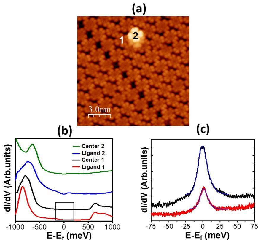
**Fig. 4.9:** (b) STM topographic image ( $V_s = -0.9$  V,  $I_T = 30$  pA) of TbPc<sub>2</sub> growth on Cu(111). (b)  $dI/dV$  spectra measured at molecule 1 (first layer) sites: Ligand (red) and center (black) and at the molecule 2 (second layer) sites: Ligand (blue) and center (green). (c) The inset in (b) shows the Kondo peaks acquired above the ligand (red) and center (black) of the molecule in the first layer with a modulation voltage of 5 mV (pp).
