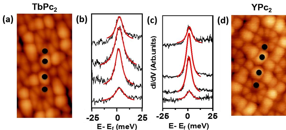
**Fig. 4.4:** (a) and (d) Topographic images STM of YPc<sub>2</sub> and TbPc<sub>2</sub> films within Phase II, showing the places (black circles) where spectroscopic data were performed on inner and outer lobes. (b) and (c) the Kondo resonances above the areas shown in the topography image in (a) and (d). data acquired with a modulation voltage of 5 mV (pp), at 4.6K, fitted by Fano function (red line).
