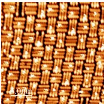
**Fig. 5.7:** High – resolution STM image showing the molecular packing in NC-Ph<sub>5</sub>-CN network with compact phase.
