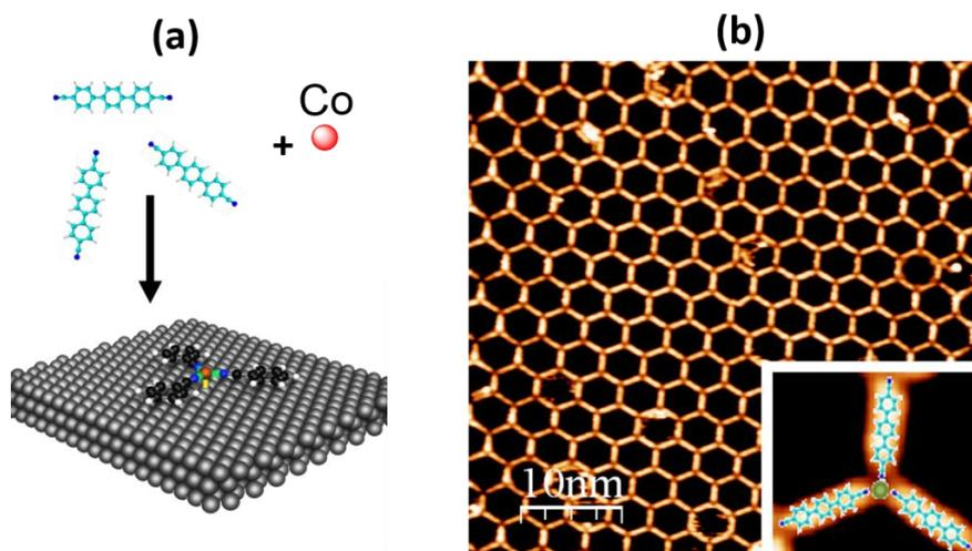
**Fig. 5.10:** (a) Simplified schematic illustrates the deposition of NC-Ph<sub>n</sub>-CN molecular linkers and the co-deposition of Co atom on the Ag(111) surface. (b) High-resolution STM image of the honeycomb network of Co (NC-Ph<sub>n</sub>-CN)<sub>3</sub> on Ag(111), the inset shows the STM topography of threefold Co(CN endgroup)<sub>3</sub> network node superimposed by corresponding templates.
