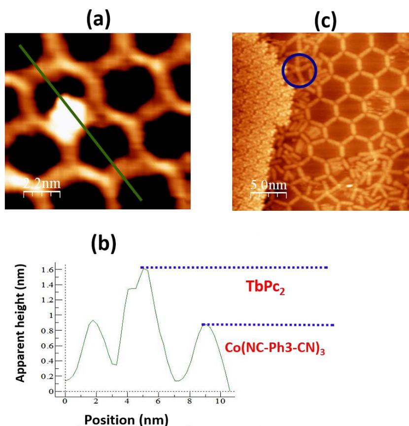
**Fig. 5.12:** High-resolution STM image of TbPc<sub>2</sub> SMM adsorption (a) on Co(NC-Ph<sub>3</sub>-CN)<sub>3</sub> and (c) on Ag(111) surface. (b) Height profile extracted along the green line in (a) shows that the TbPc<sub>2</sub> is placed above the Co (NC- Ph<sub>3</sub>-CN)<sub>3</sub> network.
