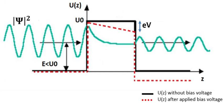
**Fig. 2.7:** Quantum regime, representation of tunneling barrier before (black line) and after (dashed red line) applied bias voltage, an electron has a certain probability to penetrate the barrier and tunnel through.
