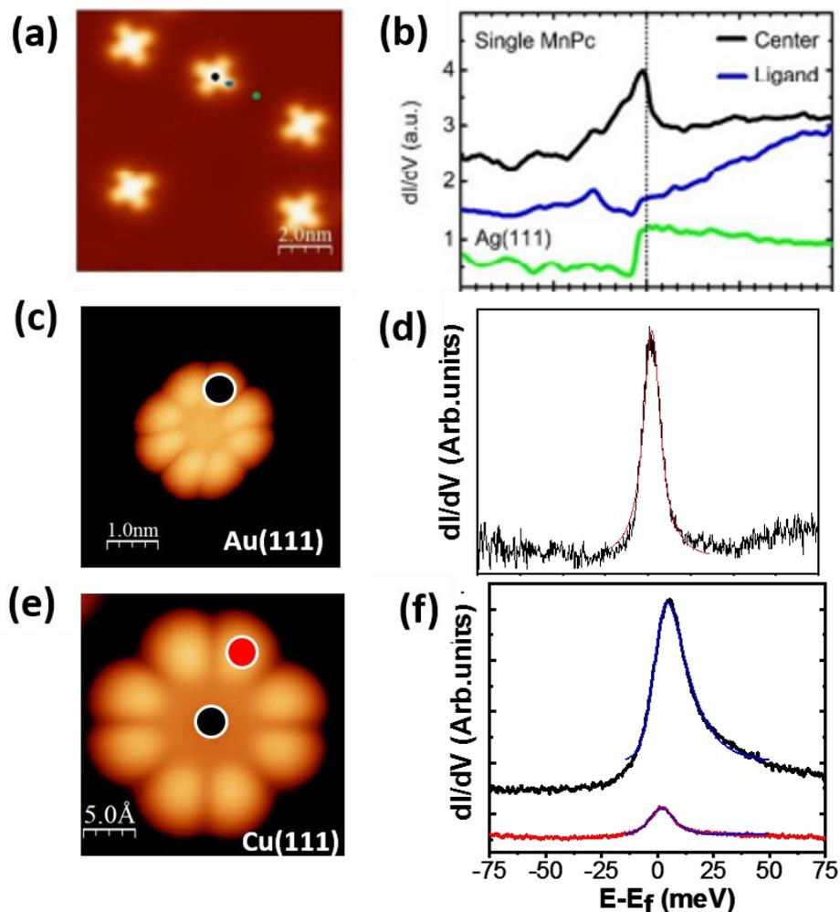
**Fig. 1.12:** (a) STM image of an MnPc molecule deposited on Ag(111). (b) dI/dV spectra on MnPc sites shows the Kondo resonance in center (extracted from [53]). (c) STM image of an isolated TbPc<sub>2</sub> molecule deposited on Au(111). (d) Kondo peak detected on the Pc ligand. (e) STM image of an isolated TbPc<sub>2</sub> molecule deposited on Cu(111). (f) Kondo peaks acquired above the ligand (red) and center (black) of the molecule.
