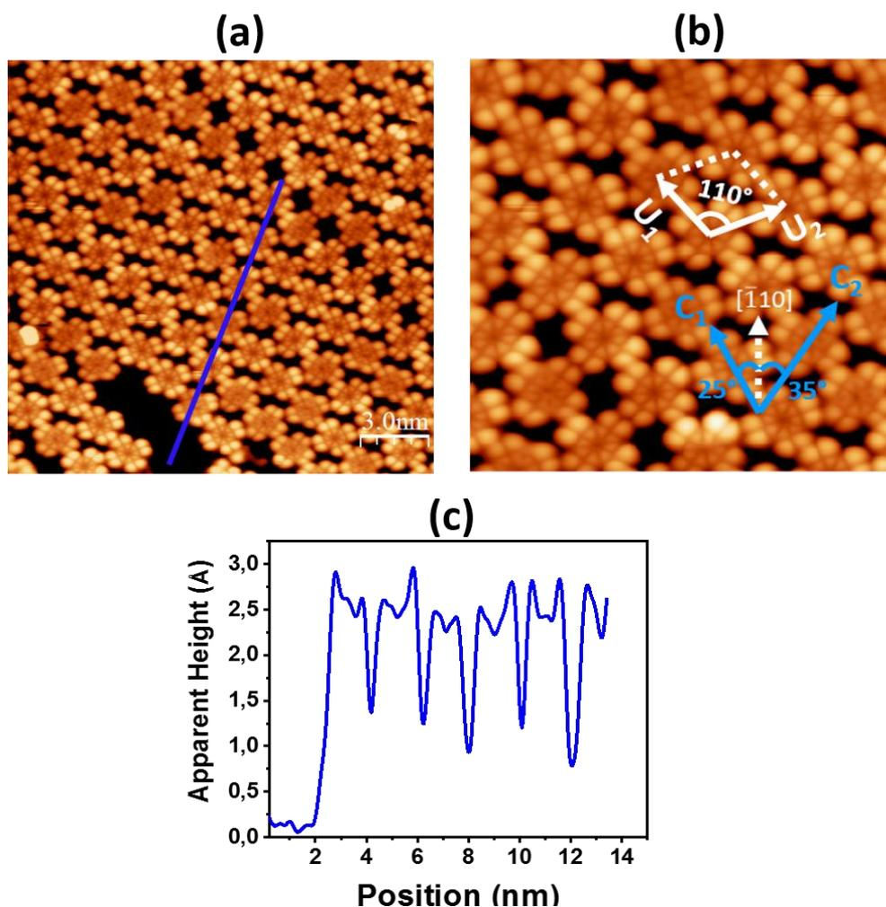
**Fig. 3.6:** (a) STM topographic images ( $V_S = -0.9$  V,  $I_T = 30$  pA) of  $TbPc_2$  growth on Cu(111). The blue line shows the adsorption profile of molecular domain growth. (b) STM topographic image of molecular domain shows the adsorption direction of  $TbPc_2$  molecules with respect of crystallographic direction of Cu(111) substrate. (c) Apparent height of Molecular domain.
