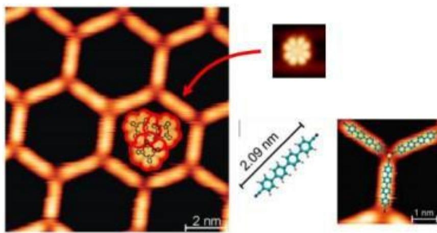
**Fig. 5.1:** Two-dimensional metal-organic network based on dicarbonitrile tetraphenyl linkers (NC-Ph<sub>4</sub>-CN) self-assembled with cobalt atoms on Ag(111) [3]. A TbPc<sub>2</sub> trimer obtained by atomic manipulation on a free surface by Amokrane et al. [5] visualized at the same scale and superposed to the original network image to show what a TbPc<sub>2</sub> trimer inside a pore would look like. The figure at the lower right shows a knot of the hexagonal network.
