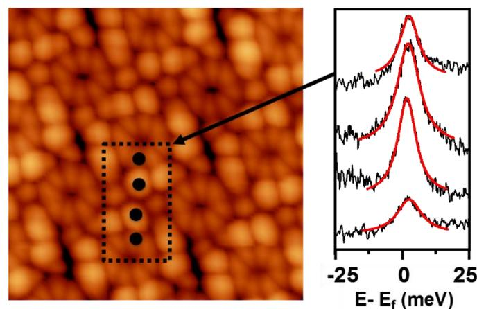
**Fig. 4.2:** Topographic STM image of TbPc<sub>2</sub> films with Phase II showing the places (marked by black circles) where spectroscopy was performed on inner & outer lobes of two adjacent
