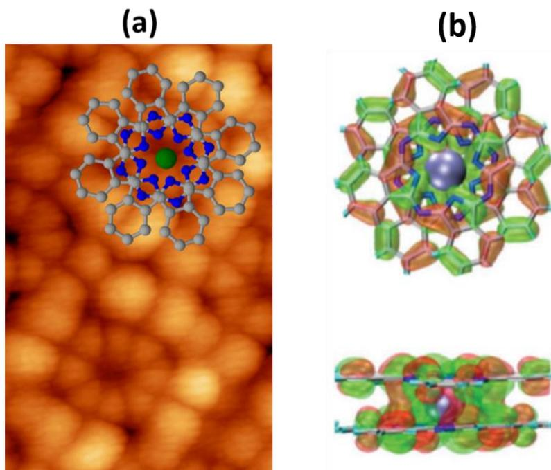
**Fig. 4.8:** (a) STM image of TbPc<sub>2</sub> domain on Au(111) with a superimposed atomic structure of TbPc<sub>2</sub>, revealing the location of the orbital of each N,C and Tb atom in the STM topographic image. (b) DFT calculation of the wave function corresponding to a spin-up state at  $-0.5$  eV evidencing the simultaneous contribution to inner and outer lobes. Red and green colors correspond to positive and negative signs of the wave function.
