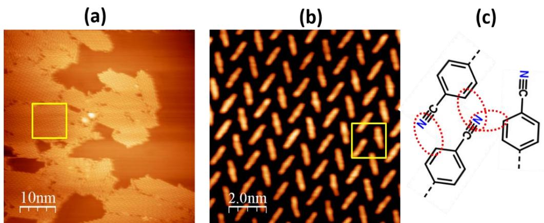
**Fig. 5.3:** (a) Topographic STM image of NC-Ph<sub>3</sub>-CN linkers self-assembled on Ag(111). (b) Yellow square in (a), High – resolution STM image showing the molecular packing with chevron phase. (c) Yellow square in (b), corresponding schematic model showing the interaction (dashed red line) between adjacent carbonitrile endgroup and phenyl groups.
