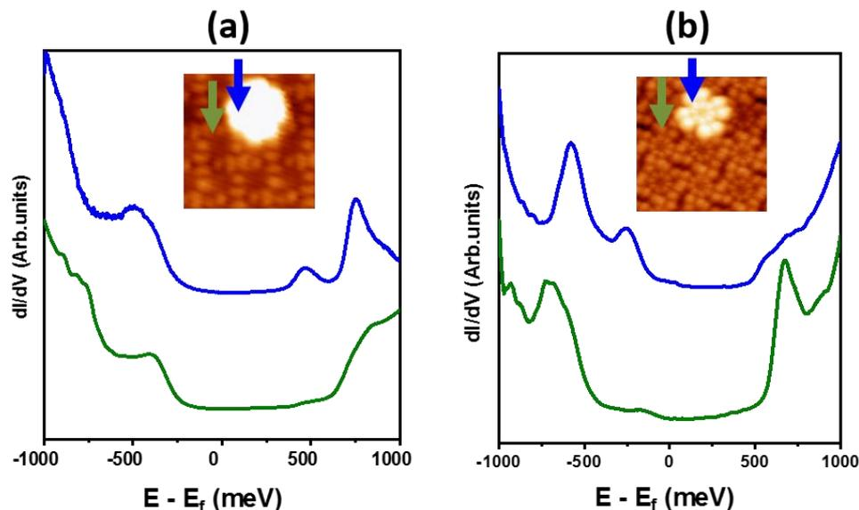
**Fig. 4.5:** dI/dV spectroscopy performed above the areas (Ligand) shown in the topography STM image (Inset) of Phase I (a) and Phase II (b), same color code. The spectra show a comparison between the HOMO/LUMO states of the TbPc<sub>2</sub> adsorbed of first- and second-layer.
