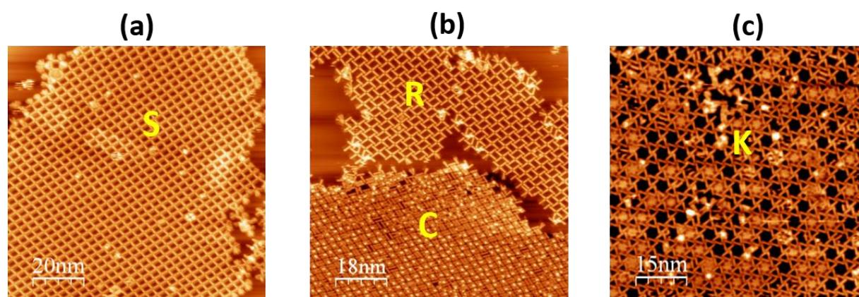
**Fig. 5.4:** Topographic STM images of NC-Ph<sub>5</sub>-CN linkers self-assembled on Ag(11) showing the molecular packing with different phases : (a) Square (S); (b) Rhombic and Compact (R and C); (c) Kagome (K).
