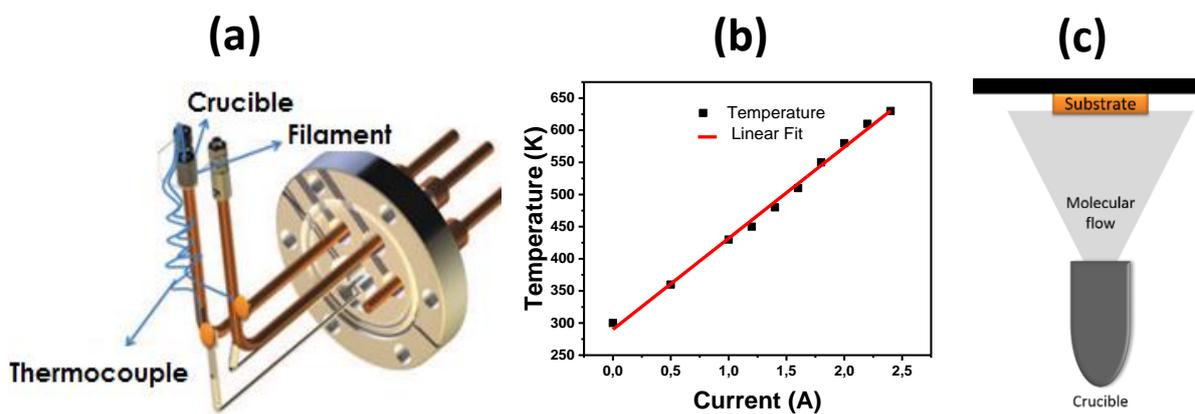
**Fig. 2.1:** (a) The home-built molecular evaporator. (b) The temperature as function of the current intensity through the filament. (c) Simplified schematic representation of the molecular evaporation procedure under UHV, The distance between the substrate and crucible is about 6 cm.
