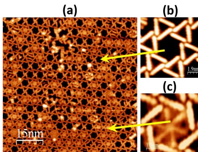
**Fig. 5.8:** (a) High – resolution STM image showing the molecular packing in NC-Ph<sub>5</sub>-CN network with Kagomé phase. (b) The empty Kagome nanopore structure on network marked by yellow alloy. (c) Molecular rotor formed by NC-Ph<sub>5</sub>-CN rotating molecules in the nanopore of the network.
