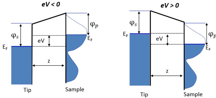
**Fig. 2.11:** Illustration of the tunneling junction between the tip and the sample when a voltage  $V$  is applied: (Left): Negative  $V$  (the electrons go from the sample to the tip); (Right): the electrons go from the tip to the sample.
