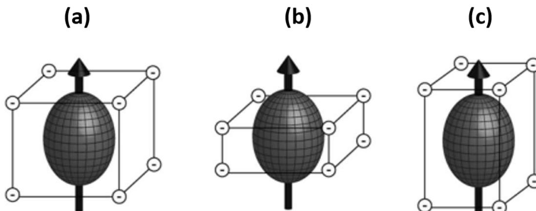
**Fig. 1.3:** The anisotropy of the 4f-shell electron distribution for tripositive lanthanides associated with the point-charge model in cubic crystal field (a) and tetragonal crystal fields (b and c).
