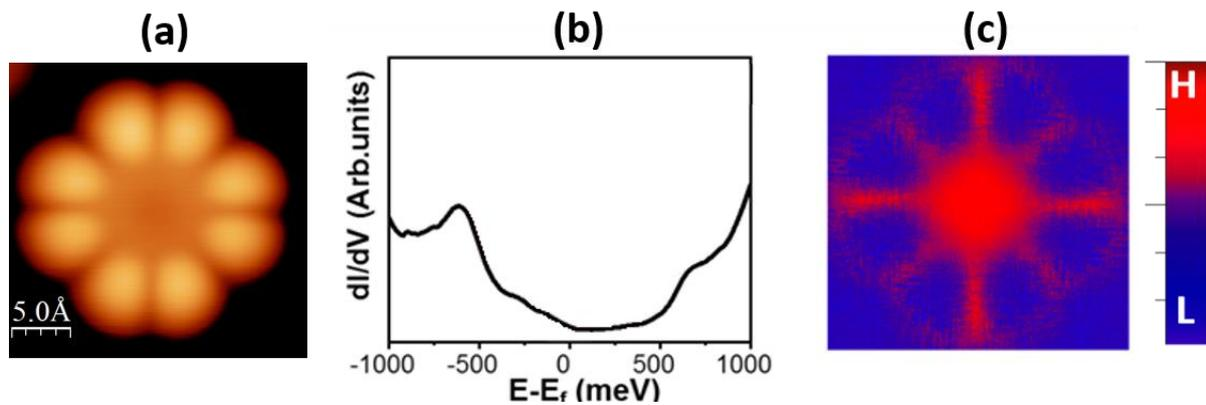
**Fig. 2.12:** Example of experimental results obtained by STM/STS on  $TbPc_2$  deposited on Cu(111). (a) Topographic STM image of  $TbPc_2$ . (b) Conductance spectrum ( $dI/dV$ ) acquired at the center revealing the HOMO and LUMO states. (c)  $dI/dV$  maps at occupied states (-0.7 V). Red: high conductance, blue: low conductance.
