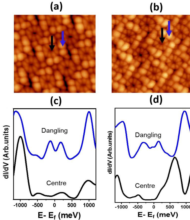
**Fig. 4.3:** (a) and (b) High resolution STM images ( $5 \times 5 \text{ nm}^2$ ) of the Phase II of TbPc<sub>2</sub> and YPc<sub>2</sub> molecular domains growth on Au(111), respectively. Blue and black arrows indicate the point where the spectra dI/dV was recorded. (c) and (d) dI/dV spectroscopy from -1.2 eV to +1.2 eV on the center and the dangling lobe of the two molecules TbPc<sub>2</sub> and YPc<sub>2</sub> as shown in (a) and (b) respectively.
