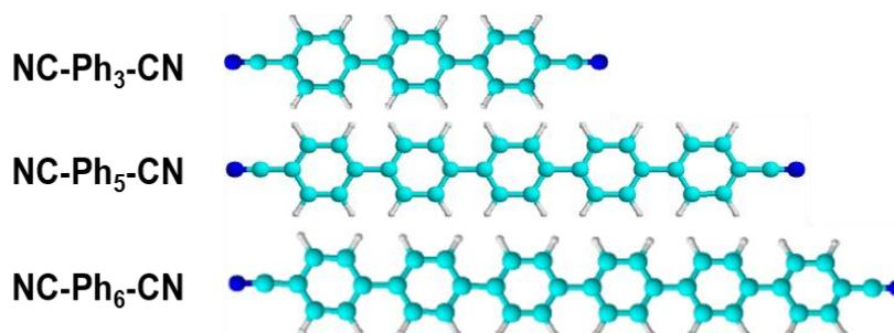
**Fig. 5.2:** Dicarbonitrile-polyphenyl Molecular structure of NC-Ph<sub>n</sub>-CN : n = 3, dicarbonitrile-terphenyl molecule (NC-Ph<sub>3</sub>-CN) ; n = 5, dicarbonitrile-pentaphenyl molecule (NC-Ph<sub>5</sub>-CN) ; n = 6 dicarbonitrile-hexaphenyl molecule (NC-Ph<sub>6</sub>-CN). Color code: Blue=Nitrogen; Cyan=Carbon; White=Hydrogen.
