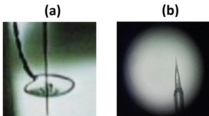
**Fig. 2.3:** Preparation method of an STM tip: (a) Electrochemical etching of a tungsten (W) piece with a NaOH solution (10%). (b) Real photo of an STM Tip.
