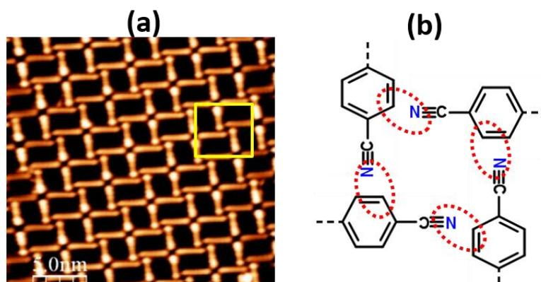
**Fig. 5.6:** (a) High – resolution STM image showing the rhombic molecular network of NC-Ph<sub>5</sub>-CN linkers. (b) Yellow square in (a), corresponding schematic model showing the interaction (dashed red line) between adjacent carbonitrile endgroup and phenyl group.
