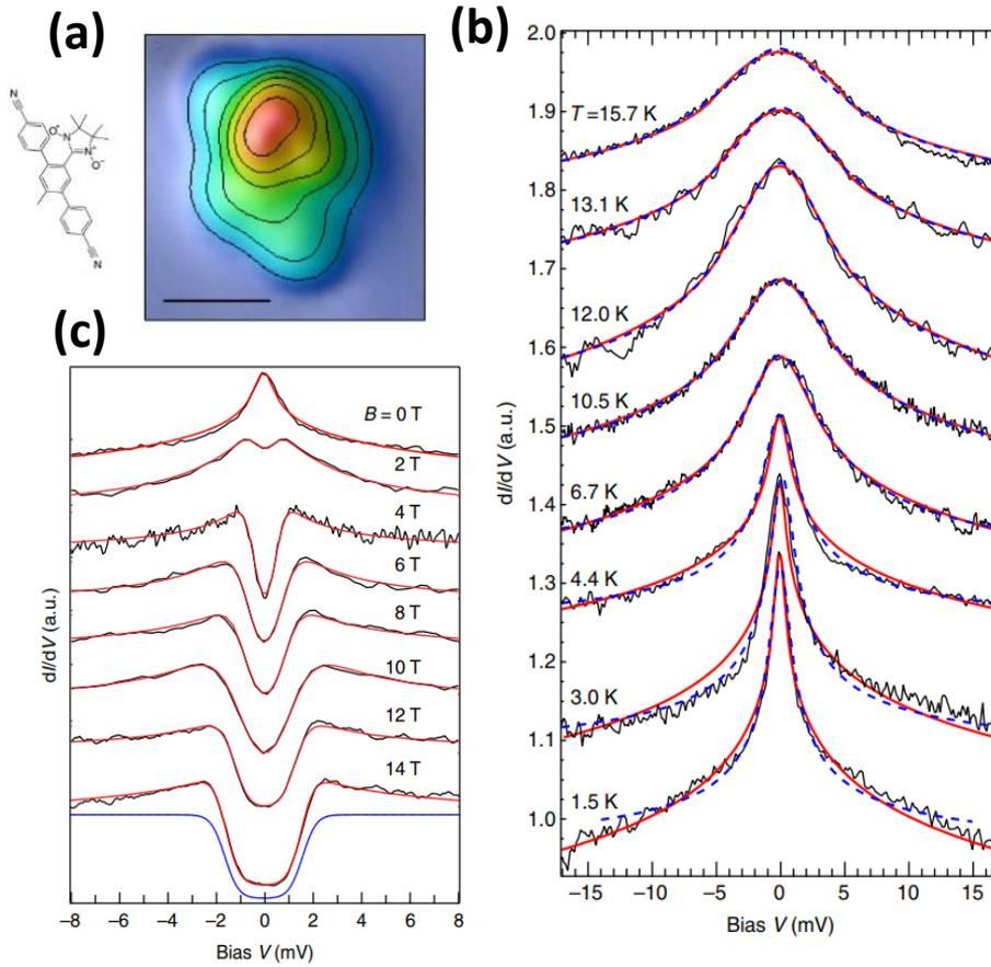
**Fig. 1.14:** (a) Chemical structure of the studied organic radical molecule ( $C_{28}H_{25}O_2N_4$ ) with a nitronyl-nitroxide side group deposited on Au(111). (b) Temperature dependence of the peaks measured in the radical side group of the molecule of 1.5–15.7K. (c) Magnetic field dependence of the peaks taken on the radical side group of the molecule. (Adapted from [55])
