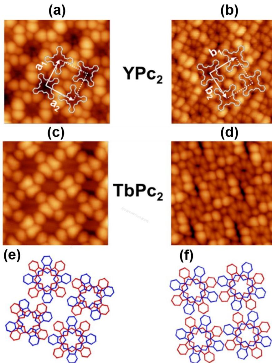
**Fig. 3.3:** STM images of molecular layers on Au(111) showing the two arrangement phases  $TbPC_2$  and  $YPC_2$  molecules in the molecular domain. (a) and (c) Phase I, image (5 nm x 5 nm) recorded at  $I_T = 90$  pA and  $V_S = -0.8$  V. (b) and (d) Phase II, image (5 nm x 5 nm) recorded at  $I_T = 90$  pA and  $V_S = -1$  V. Schematic models for the unit cells showing the upper Pc's (Blue) and bottom Pc's (red) for (e) Phase I and (f) Phase II.
