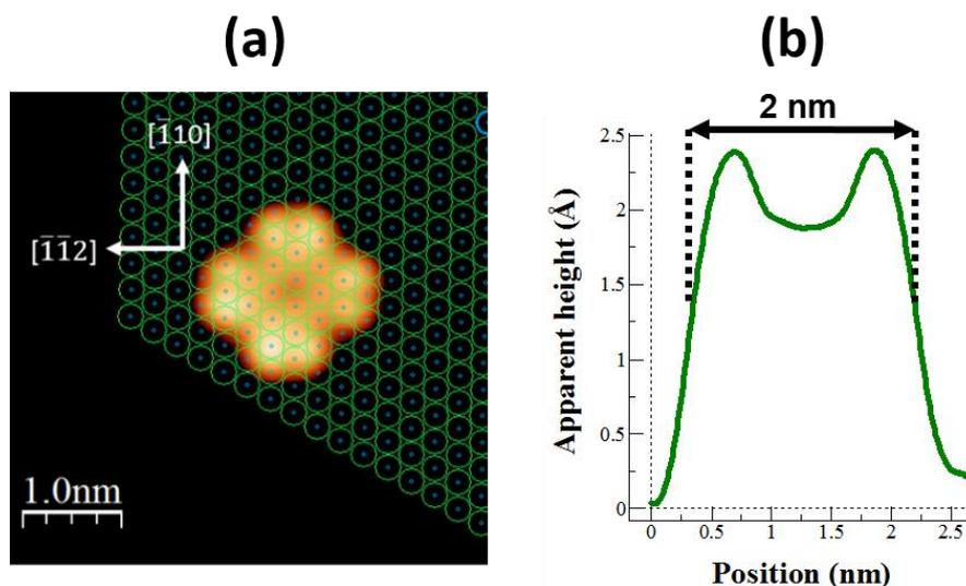
**Fig. 3.5:** (a) STM topographic image of an individual  $TbPc_2$  on Cu(111) obtained at ( $V_S = 0.7$ ,  $I_T = 20$  nA), the molecular axes are aligned with the high symmetry and directions of the Cu(111). (b) Apparent height of the individual  $TbPc_2$  molecule adsorbed on Cu(111).
