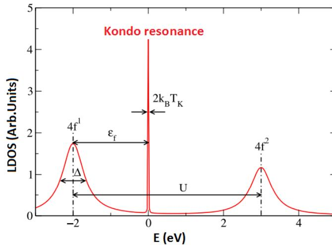
**Fig. 1.9 :** Simulation of LDOS of the cerium impurity. The half-width at half height is worth  $k_B T_K \equiv \Gamma$ . The parameters used for the calculation are  $\epsilon_F = -2$  eV,  $U = 5$  eV,  $\Delta = 0.34$  eV, (Adapted from [45])
