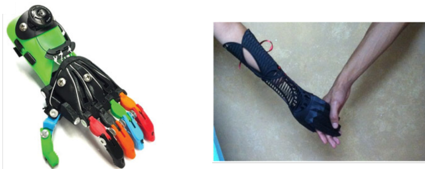
Figure 1.8: Examples of personalized 3D-printed UL prostheses, from [40], body-powered (left) and esthetic (right)
