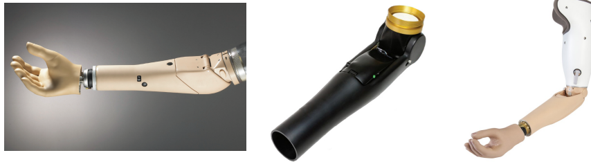
Figure 1.7: Commercialized elbow prostheses. From left to right: Utah Arm (from [38]), Boston Arm (from [39]) and Dynamic Arm (from [21])
