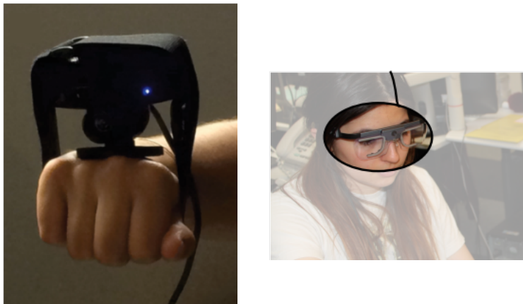
Figure 2.6: Examples of in-hand camera, from [134] (left) and cameras on glasses, from [104] (right)
