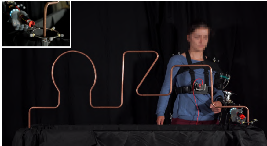
Figure 3.9: Cybathlon wire-loop task with the emulated prosthetic device. The upper left insert shows the handle hold by the prosthetic hand.
