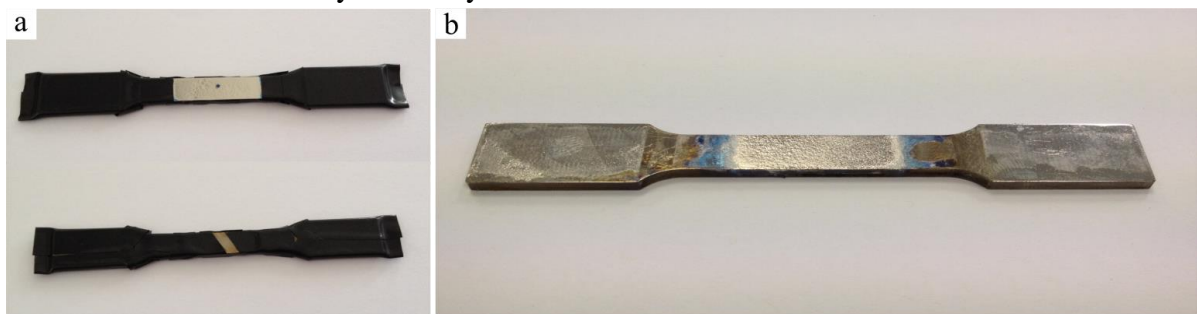
Fig. 3-11. Particular protected tensile test sample for electrolytic polishing: (a) the protection; (b) the final sample after electrolytic polishing.
