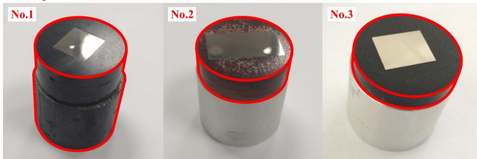
Fig. 3-14. Three IIT samples of different self-weights.
