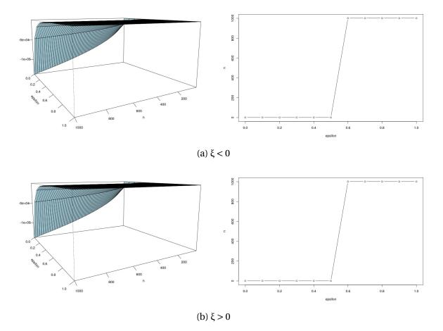
Figure 4.20 – Representation of both utility function  $U_{t_r}(n)$  (on left side), and  $n^*$  (on right side) according to the variation of parameter  $\epsilon$  ( $\epsilon = \{0, 0.1, 0.2, ..., 1\}$ ), with biased expectations.
