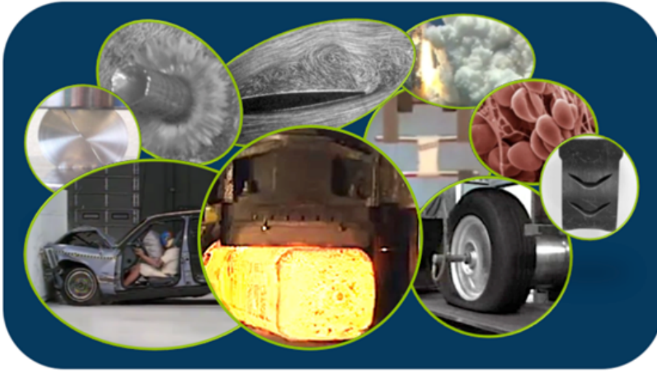
Figure 1.1: Examples of large transformations of matter. Clockwise starting with the center: forging process, crash test, rupture of a disk, shot impact, turbulence due to an airplane wing, gas explosion, tensile test of vessel replacement, deformed red blood cells, defects in an extruded metallic part, fatigue test of a tire.
