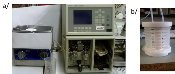
Figure 2. a. A photograph of millifluidic system b. A photograph of the reactor with Teflon tubing.
