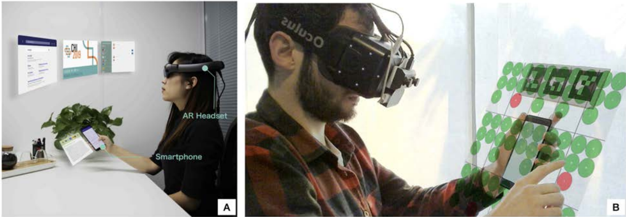
Figure 2.21: (A) Understanding window management interactions using an AR-HMD + smartphone interface [23]. (B) Enlarging smartphone display with an AR-HMD [112].
