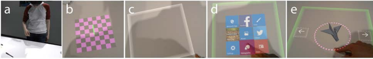
Figure 2.4: MRTouch enables touch interaction in AR-HMDs [72]. (a) When a user approaches a surface, MRTouch detects the surface and (b) presents a virtual indicator. (c) The user touch-drags directly on the surface to (d) create a launcher and start an app. (e) In this app, the user uses touch to precisely rotate a 3D model.
