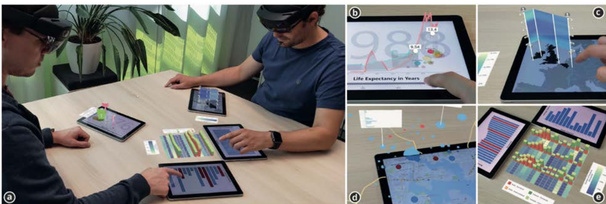
Figure 2.22: Data visualization using mobile devices and Augmented Reality head-mounted displays [113]: (a) Envisioned usage scenario; (b) 2D scatter-plot extended with superimposed 3D trajectories/paths; (c) 3D wall visualization in AR aligned with the mobile device; (d) Use of AR for seamless display extension around a geographic map; (e) Combining visualizations with an AR view between the devices.
