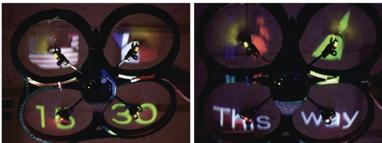
Figure 4.10: ARial Texture tracks the position and orientation of a drone and projects a texture on the drone's propellers accurately [206].
