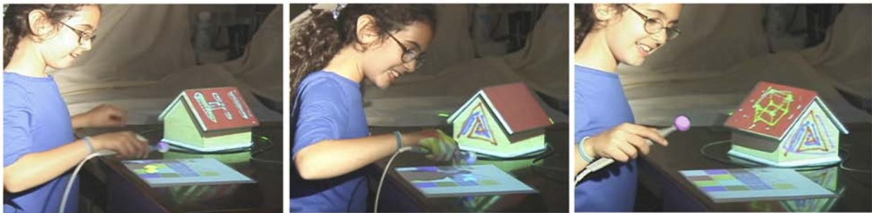
Figure 2.29: Dynamic shader lamps for applying virtual paint and textures to real objects simply by direct physical manipulation of the object and a “paint brush” stylus. [31].
