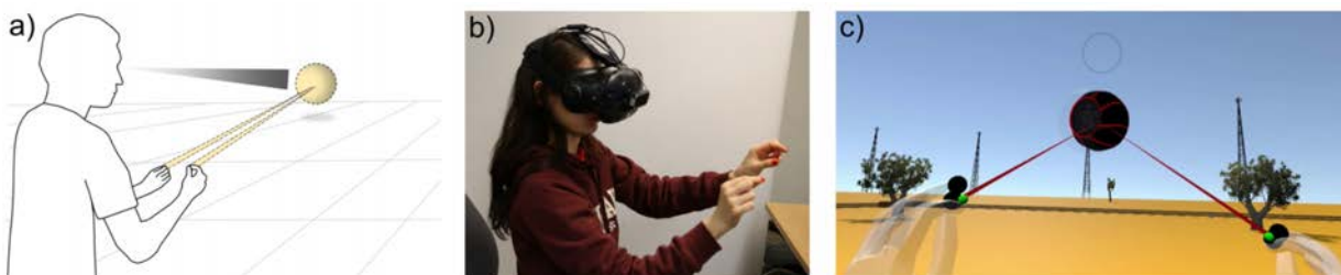
Figure 2.25: Gaze + Pinch interactions unify a user's eye gaze and hand input: look at the target, and manipulate it (a); virtual reality users can utilise free hand direct manipulation (b) to virtual objects at a distance in intuitive and fluid ways (c).
