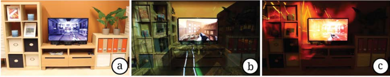
Figure 1.6: IllumiRoom is a proof-of-concept system that augments the physical environment surrounding a television to enhance interactive experiences [53]. (a) With a 3D scan of the physical environment, we can (b) directly extend the FOV of the game, (c) selectively render scene elements.
