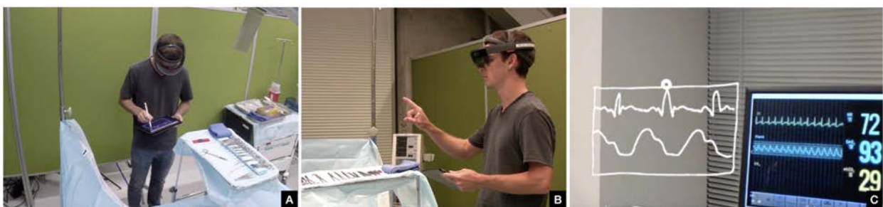
Figure 2.16: PintAR [108] in use. (A) Designer sketching an interface element on the tablet using a pen. (B) Designer placing sketched element in the environment using an Air tap. (C) AR interface element placed side-by-side with real display.
