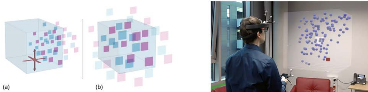
Figure 2.23: Left: 3D data spaces can be explored by (a) 3D panning and (b) zooming relative to their fixed presentation space. Right: A user wearing a HoloLens explores such a 3D data space with smartphone-based proposed interaction techniques [19].
