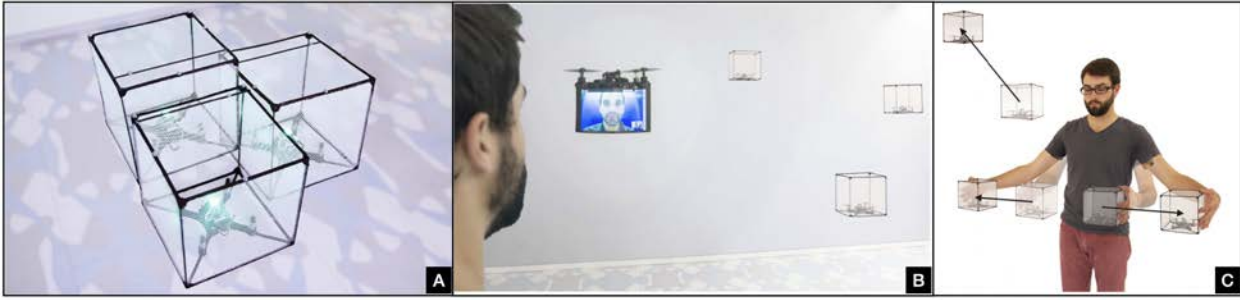
Figure 4.11: (A) BitDrones [210] hovering in a tight formation. (B) User inspecting a remote facility with telepresence functionality provided by the drone. (C) User resizing a compound object using a bi-manual pinch gesture by moving drones.
