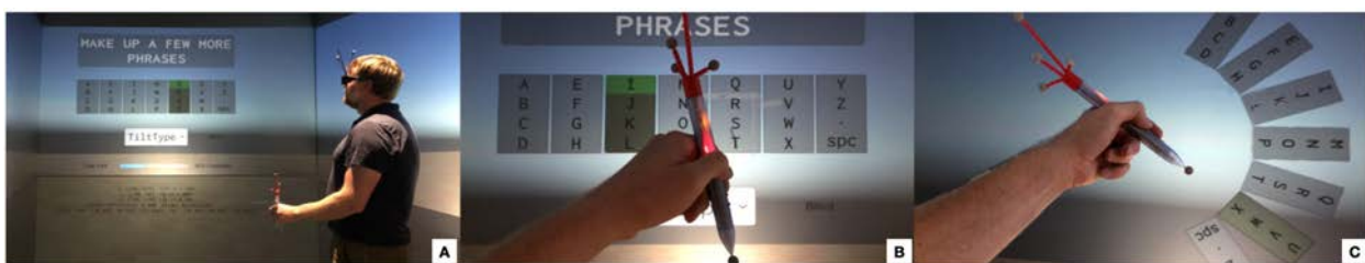
Figure 2.18: (A) The overall setup of a stylus-based text input system in a CAVE environment [111]. (B) The Tilt-Type interface. (C) The Arc-Type interface.
