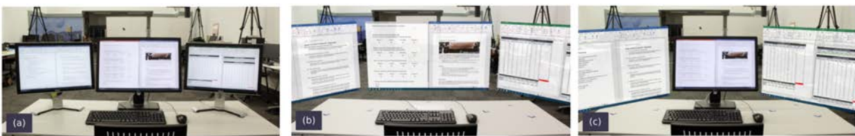
Figure 1.1: Comparing physical monitors, virtual AR monitors, and a hybrid combination of both for productivity tasks [36]: (a) Physical condition had three monitors side-by-side; (b) Virtual condition had three monitors rendered through HoloLens; (c) Hybrid condition combined a central physical monitor with two peripheral virtual monitors.
