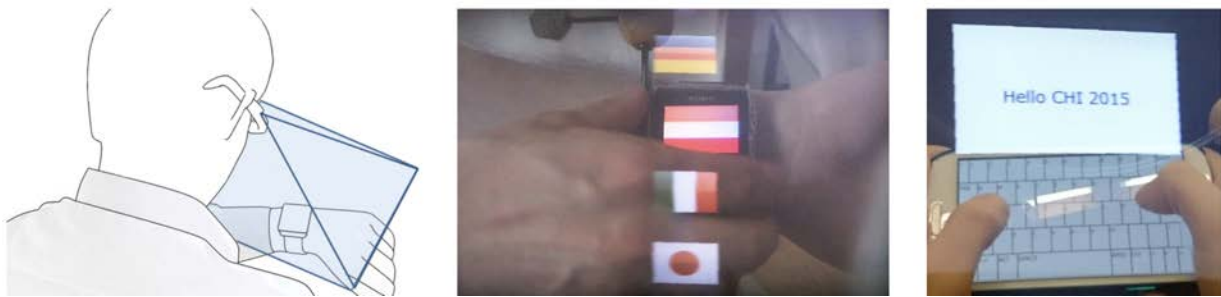
Figure 2.19: MultiFi [21] widgets crossing device boundaries based on proxemics dimensions (left), e.g., middle: ring menu on a smartwatch (SW) with head-mounted display (HMD) or right: soft keyboard with full-screen input area on a handheld device and HMD.
