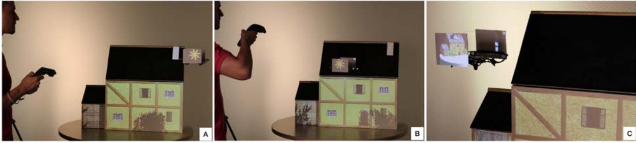
Figure 4.14: (A - B) The light source of our scene is at the drone hovering position. By moving the light source, the user is casting shadows on the scene. (C) An interactive 3D model of the mock-up displayed next to the physical one allows the user to observe the scene from another viewpoint.
