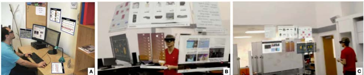
Figure 1.3: (A) In an AR workspace, virtual windows are embedded into the user's nearby surfaces [38]; (B & C) AR interfaces adapt dynamically based on the user's walking and physical environment [41].
