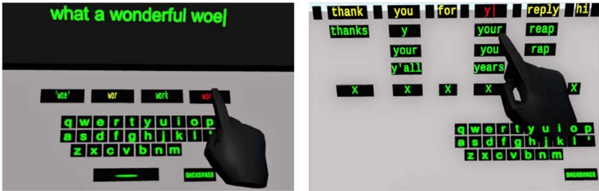
Figure 2.24: Typing on a midair auto-correcting keyboard with word predictions (left) vs. speaking a sentence and then correcting any speech recognition errors (right) [127]. Users correct errors by selecting word alternatives proposed by the speech recognizer or by typing on the virtual keyboard.
