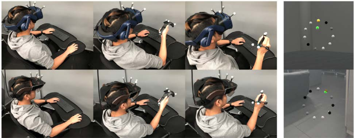
Figure 2.14: Pointing tasks in VR (top) and AR (bottom) using a mouse, a VR controller, and a 3D pen [106].
