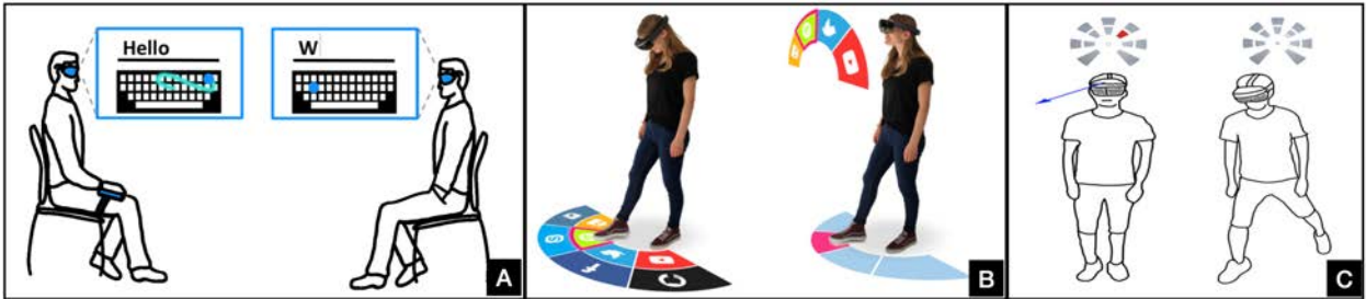
Figure 2.13: (A) Word-gesture and tap based typing around the thigh [97]. (B) Foot-taps as a direct and indirect input modality for interacting with HMDs [98]. (C) A user needs to go the North-East direction using DMove technique and a selection is made when the user (nearly) completes the action [16].
