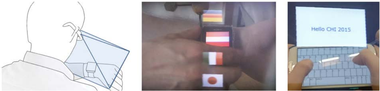
Figure 2.19: MultiFi [21] widgets crossing device boundaries based on proxemics dimensions (left), e.g., middle: ring menu on a smartwatch (SW) with head-mounted display (HMD) or right: soft keyboard with full-screen input area on a handheld device and HMD.
